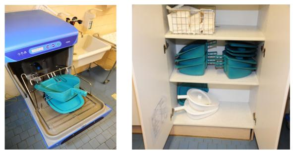
Fig. 11-7: Bedpan and urinal bottle washer and storage closet
