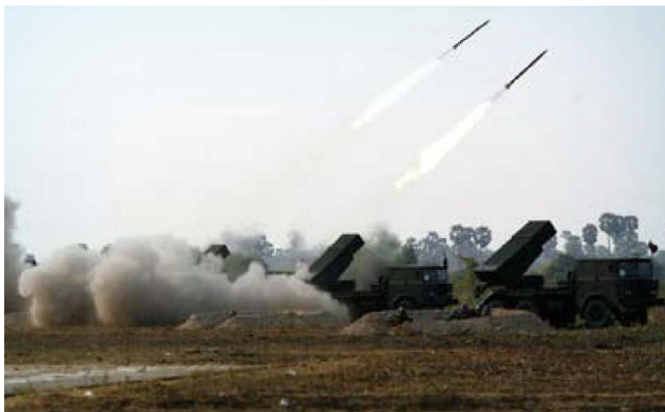
Photo 5. An example of the visual launch signature from multiple 122 mm MBRL firing; in this case, Chinese Type 81 variants (Photo credit: Xinhua/Reuters Photo).
