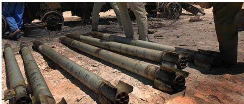
Photo 6. Grad rocket fins in the open position (Photo credit: Sean Sutton/MAG).
