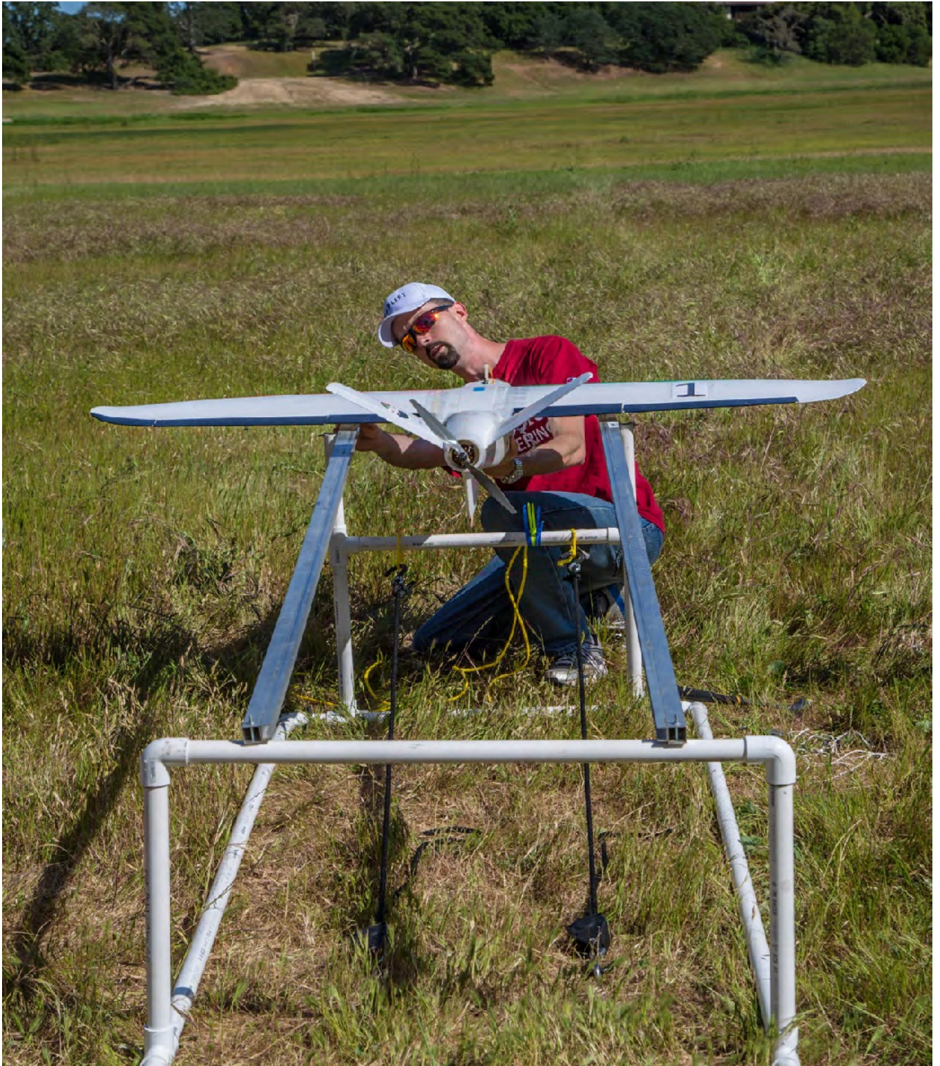
Figure 4-1 Michael Taylor, with Uplift Aeronautics' Waliid drone mounted on a home-built PVC launcher
