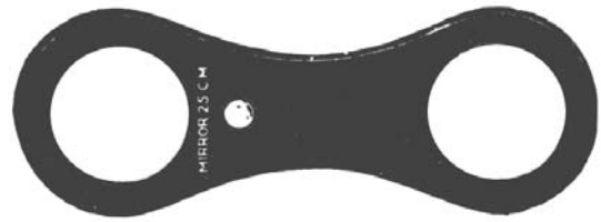
Fig. 7.2: Retinoscope—plano and concave mirrors
