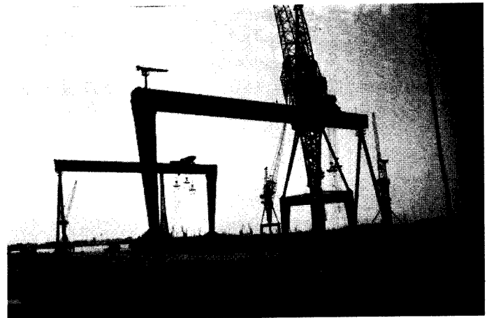
Figure 26.67 Building Dock Gantry Cranes
