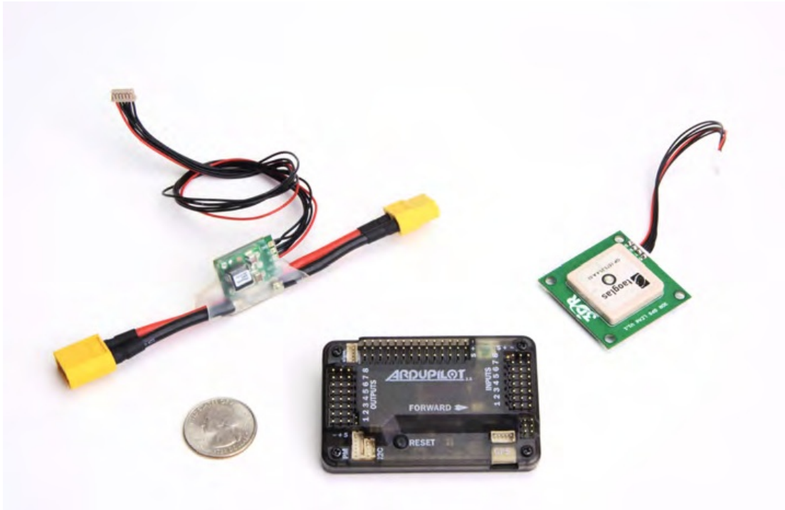
Figure 2-3 An ArduPilot flight controller with power monitor and GPS
