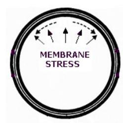
devoid of abrupt inside corners or pockets that promote localized fluid stagnation. Structurally, the curved shell produced by the circular pipe cross section allows a multiplicity of alternative stress paths and gives the optimum form for transmission of many different load types. This holds true for both internal loads like pressure and external loads such as those produced by back fill material or internal vacuum conditions. The single curvature allows for a
