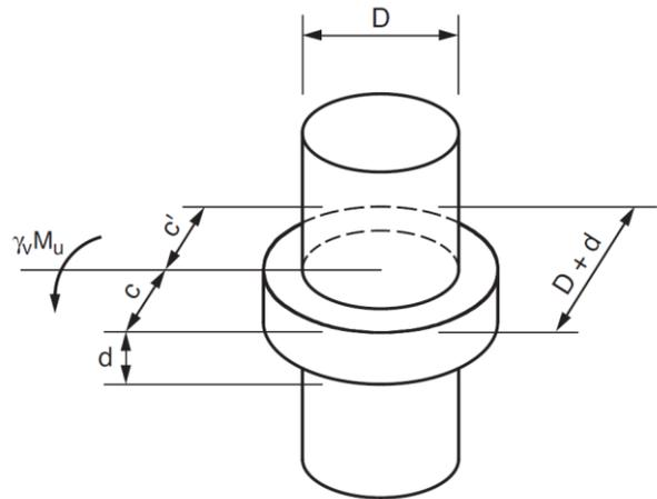
Excerpt from Fig. 16-14 of PCA Notes on ACI 318-11<sup>[9]</sup> where  $D$  equals to the diameter of circular column,  $h_c$
