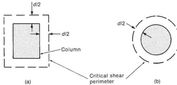
Location of critical shear perimeter – Excerpt from pg. 689 of Reference [10]
