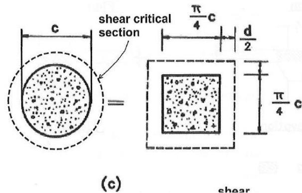
Excerpt from Fig. 3.1b of ACI 352.1R-11<sup>[8]</sup> where  $c$  equals to the diameter of circular column,  $h_c$ .
