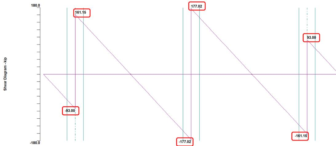
Shear Force Diagram from [spSlab](#)
