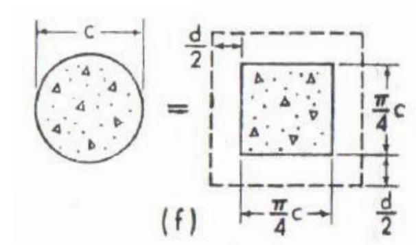
Excerpt from Fig. 7 of ACI-ASCE Committee 426<sup>[3]</sup> where  $c$  equals to the diameter of circular column,  $h_c$ .
