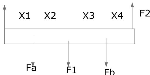
$$X_1 = 4\text{m}, X_2 = 2\text{m}, X_3 = 1\text{m}, X_4 = 1\text{m}, F_a = 10\text{ N}, F_b = 30\text{ N}$$
