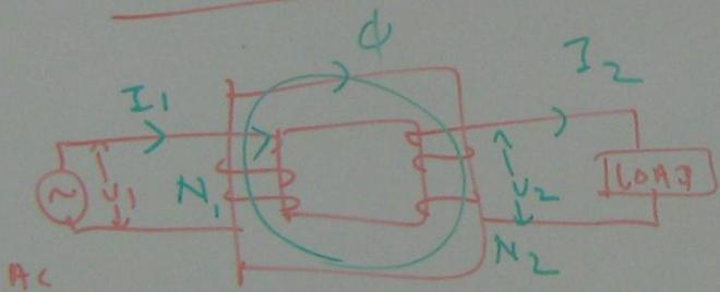
$$\frac{N_1}{N_2} = \frac{V_1}{V_2} = \frac{I_2}{I_1} = a$$
