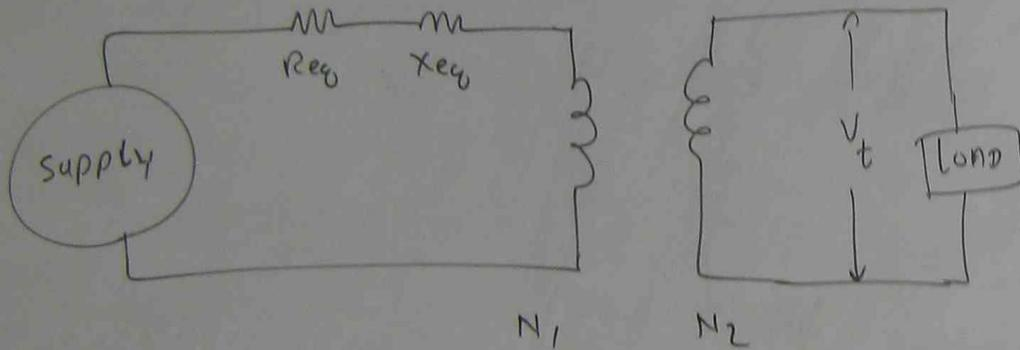
LAGGING P.F  $\Rightarrow$   $\% \text{ VOLTAGE REGULATION} = \frac{I_s' (R_{eq}' \cos\theta + X_{eq}' \sin\theta)}{V_p} \times 100$
