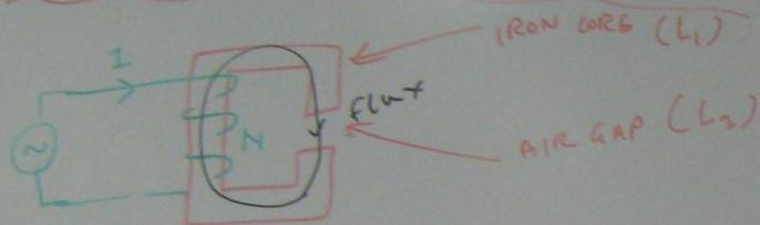
$$\begin{aligned} \text{MAGNETO force} &= \text{CURRENT} \times \text{NO. OF TURNS} \\ &= I \times N \\ &= NI \end{aligned}$$
