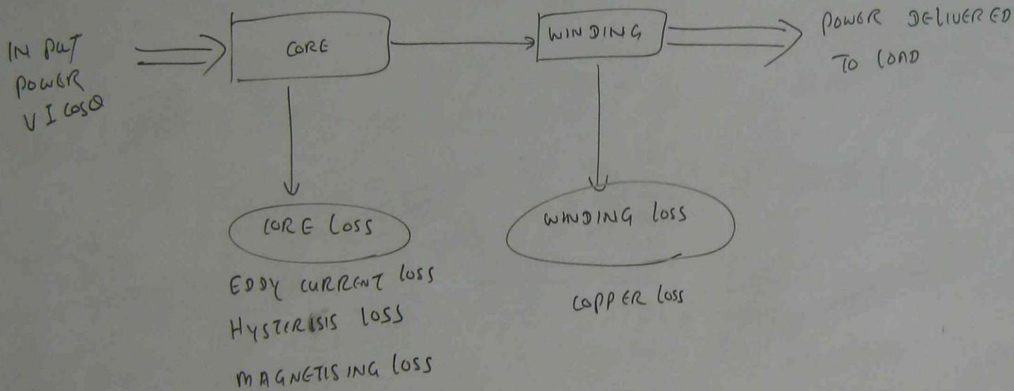
$$\% \text{ EFFICIENCY} = \frac{\text{INPUT POWER} - (\text{CORE LOSS} + \text{WINDING LOSS})}{\text{INPUT POWER}} \times 100$$
