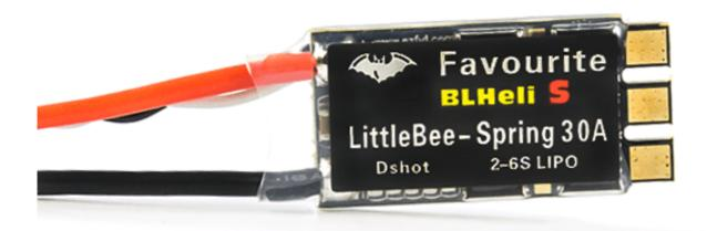
ESC's are available to purchase individually or as a 4-in-1 PCB. A 4-in-1 saves weight, and is convenient to build it into the stack, It also centralizes the mass of the quad which will improve responsiveness. ESC's can be prone to failure, so using individual ESC's means you can swap one out if needed.
