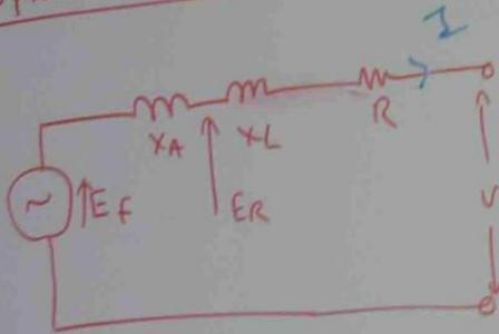
$X_A$  = SERIES CONNECTED REACTANCE OF VOLTAGE WINDING
