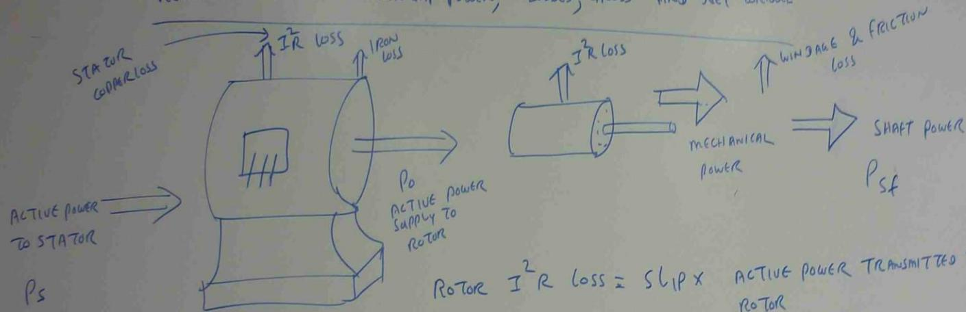
$$\begin{aligned} \text{ROTOR } I^2 R \text{ LOSS} &= \text{SLIP} \times \text{ACTIVE POWER TRANSMITTED TO ROTOR} \\ &= \text{SLIP} \times P_o \end{aligned}$$
