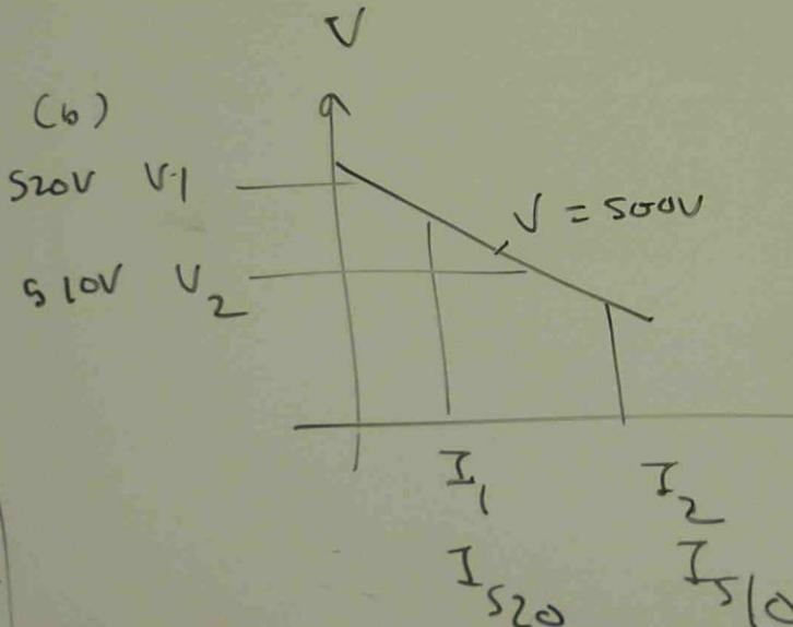
$$\frac{V_1 - V_2}{V_1 - V} = \frac{I_2}{I_1}$$
