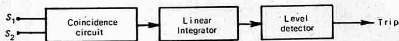
FIGURE 11.18 Block schematic for integration of coincidence blocks.
