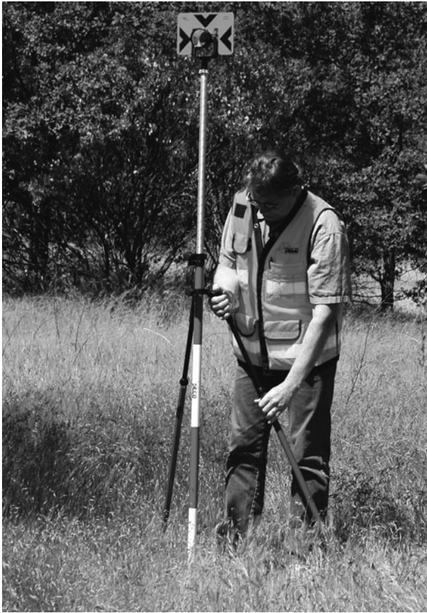
FIGURE 3.29 Steadying the EDM reflector by using a bipod. (Courtesy of SECO Manufacturing, Redding, CA. Photo by Eli Williem)
