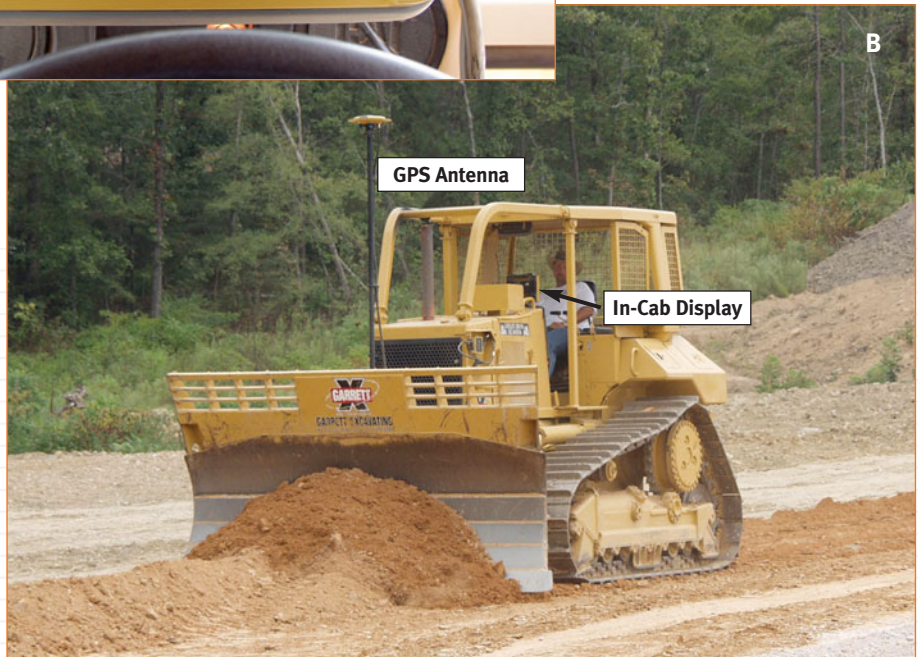
GPS machine guidance and control. (a) In-cab display. The Topcon System 5 3D in-cab display/control panel features touch-screen operation and the ability to monitor the position of the controlled equipment over the entire job site in multiple views. (b) GPS-controlled bulldozer. Rough grading is performed by a bulldozer equipped with a Topcon 3D-GPS+ control system without any need for grade stakes. (Courtesy of Topcon Positioning Systems, Inc., Pleasanton, Calif.)
