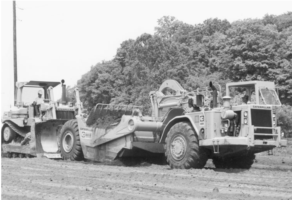
FIGURE 12.16 Scraper (shown being assisted by a bulldozer) used for efficient transfer of cut material to fill areas. (Courtesy of Caterpillar, Inc.)
