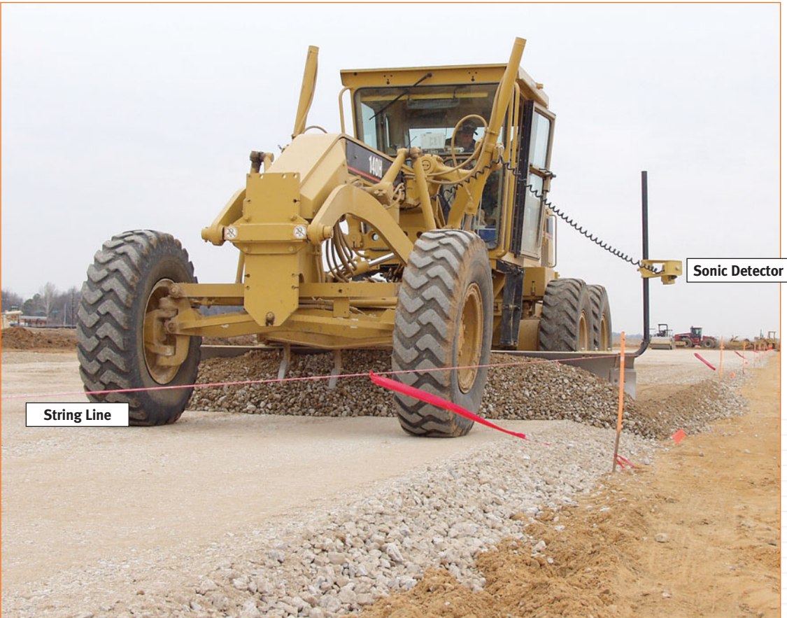
Sonic detection machine guidance. This conventional machine guidance system uses a high-accuracy sonic transmitter to locate a string (or wire) set to proper grading specifications. (Courtesy of Topcon Positioning Systems, Inc., Pleasanton, Calif.)
