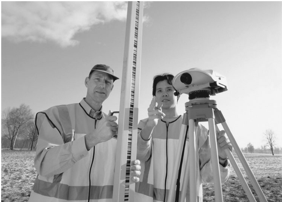
FIGURE 2.7 DNA03 digital level and bar-code rod. (Courtesy of Leica Geosystems)
