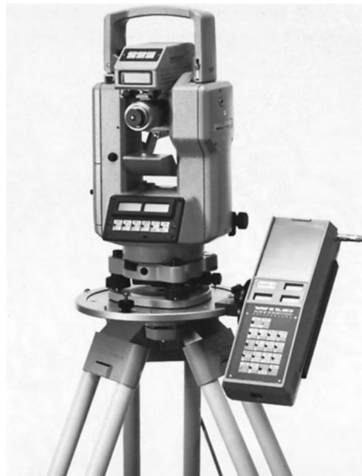
FIGURE 3.24 Wild T-1000 electronic theodolite, shown with DI 1000 Distomat EDM and the GRE 3 data collector. (Courtesy of Leica Geosystems)
