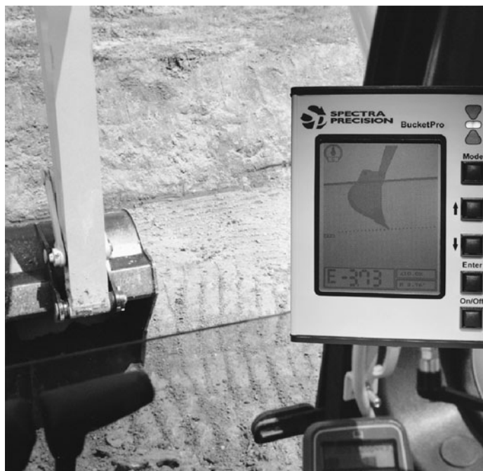
FIGURE 10.2 BucketPro Excavator cab display system used in machine-controlled excavation. The screen display shows the bucket teeth in relation to the proposed gradient. (Courtesy of Trimble Geomatics and Engineering Division)
