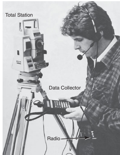
FIGURE 1.6 Sokkia total station.
