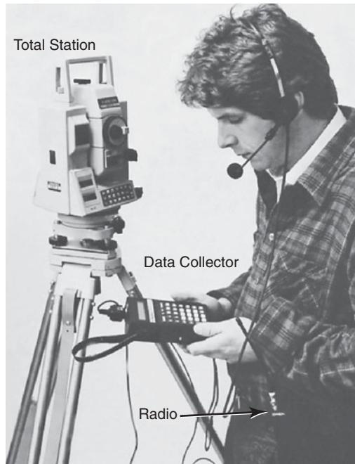
FIGURE 5.3 Sokkia total station with cable-connected electronic field book. Also shown is a two-way radio (2-mi range) with push-to-talk headset.
