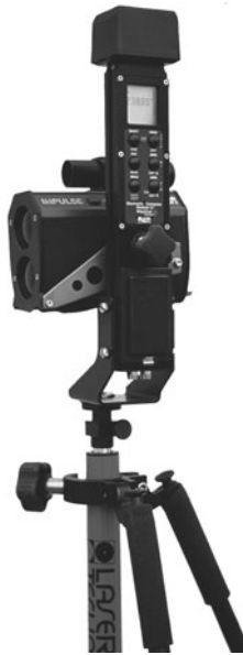
FIGURE 7.22 MapStar Compass Module II, which has reflectorless EDM capabilities and azimuth determination (accuracy of \pm 0.6^\circ ). (Courtesy of Laser Technology Inc., Englewood, Centennial, Colorado)
