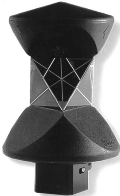
FIGURE 5.23 Leica 360° prism—used with remote-controlled total stations and with automatic target recognition (ATR) total stations. ATR eliminates fine pointing and focusing. The 360° feature means that the prism is always facing the instrument. (Courtesy of Leica Geosystems Inc.)
