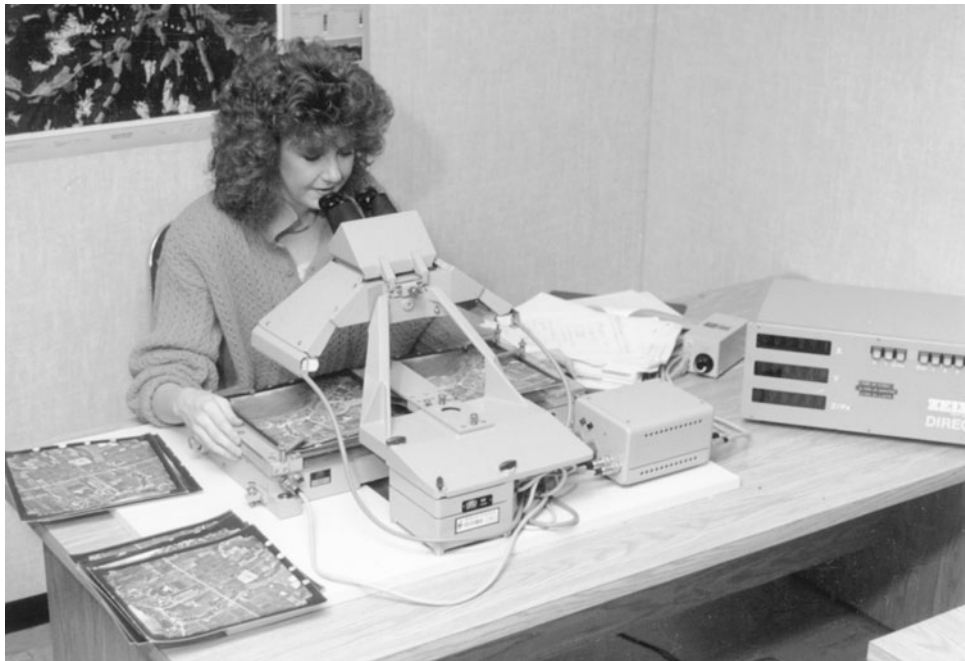
FIGURE 12.1 Zeiss G-2 Stereocord. Stereo-paired aerial photos are analyzed with horizontal and vertical data digitized for later plotting and analysis.
