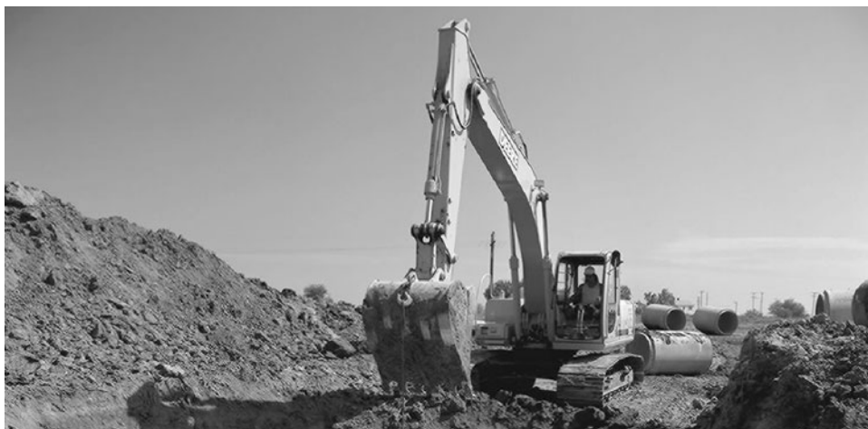
FIGURE 14.9 John Deere 792 Excavator, shown installing concrete sewer pipe. (Courtesy of John Deere, Moline, Illinois)
