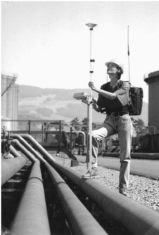
FIGURE 7.3 Leica SYS 300. System includes the following: SR 9400 GPS single-frequency receiver, with AT 201 antenna, and CR333 controller, which collects data and provides software for real-time GPS. It can provide the following accuracies: 10–20 mm +2 ppm using differential carrier techniques; and 0.30–0.50 m using differential code measurements. (Courtesy of Leica Geosystems, Inc.)
