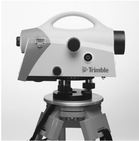
FIGURE 9.4 Precise level. Precise optical levels have accuracies in the range of 1.5–1.0 mm for 1-km two-way leveling—depending on the instrument model and the type of leveling rod used. See also Figure 2.7. (Courtesy of Trimble)
