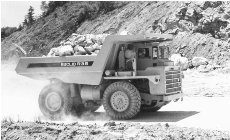
FIGURE 12.17 Euclid R35 hauler, capacity of 30.5 cu. yd. (Courtesy of Euclid-Hitachi Heavy Equipment, Ltd.)
