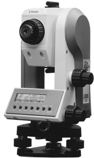
FIGURE 3.23 Trimble total station. The Trimble 3303 total stations incorporate DR technology (no prism required) and include the choice of the integrated Zeiss Elta control unit, detachable Geodimeter control unit or handheld TSCe data collector, and a wide range of software options. (Courtesy of Trimble Geomatics & Engineering Division, Dayton, Ohio)
