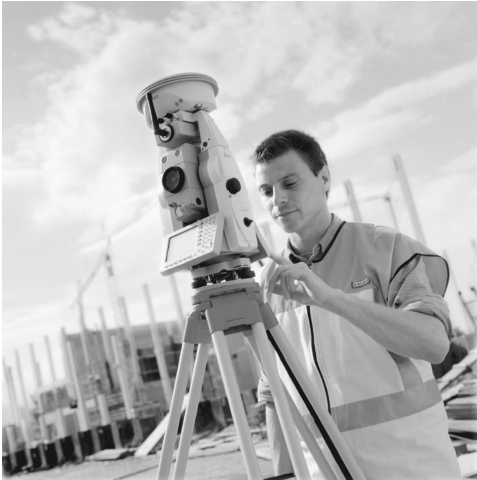
FIGURE 5.29 Leica SmartStation total station with integrated GPS. (Courtesy of Leica Geosystems Inc.)
