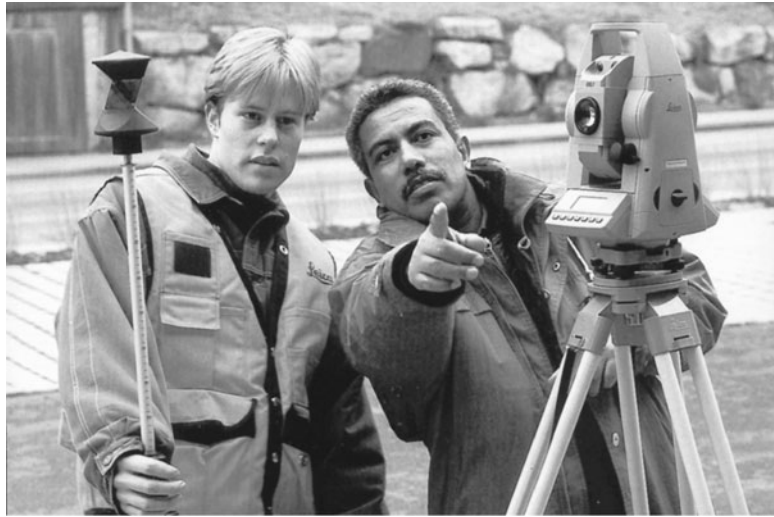
FIGURE 5.21 Leica TC 800 total station with electronic guide light. (Courtesy of Leica Geosystems Inc.)
