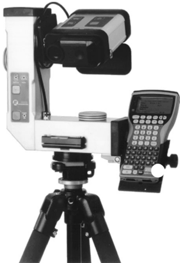
FIGURE 5.30 The reflectorless total station is equipped with integrating distance measurement, angle encoding, and data collection. (Courtesy of Riegl USA Inc., Orlando, Florida)
