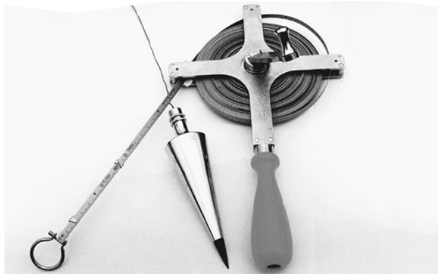
FIGURE 3.3 Steel tape and plumb bob.
