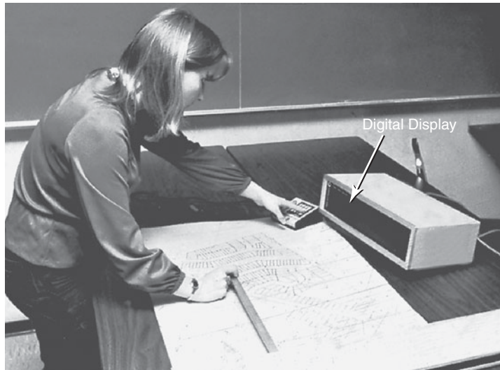
FIGURE 17.11 Area takeoff by an electronic planimeter.
