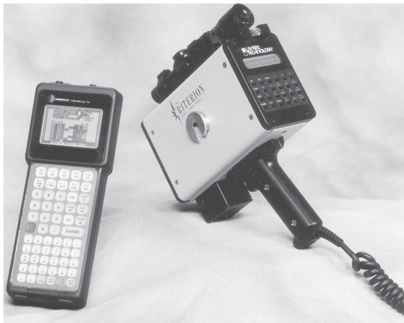
FIGURE 7.23 (a) Criterion hand-held survey laser (300), with data collector; angles by fluxgate compass; distance without a prism to 1,500 ft (to 40,000 ft with a prism). This instrument is used to collect data with an accuracy of \pm 0.3^\circ and \pm 0.3 ft for mapping and GIS databases. It provides a good extension to canopy-obstructed GPS survey points. (Courtesy of Laser Technology Inc., Englewood, Colorado).
