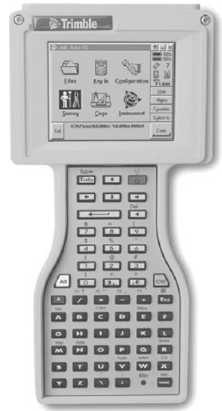
FIGURE 5.15 Trimble's TSCe data collector for use with robotic total stations and GPS receivers. When used with TDS Survey Pro Robotics software, this collector features real-time maps, 3D design stakeout, and interactive DTM with real-time cut-and-fill computations. When used with TDS Survey Pro GPS software, this collector can be used for general GPS work, as well as for RTK measurements at centimeter-level accuracy. (Portions © 2001 Trimble Navigation Limited. All Rights Reserved)
