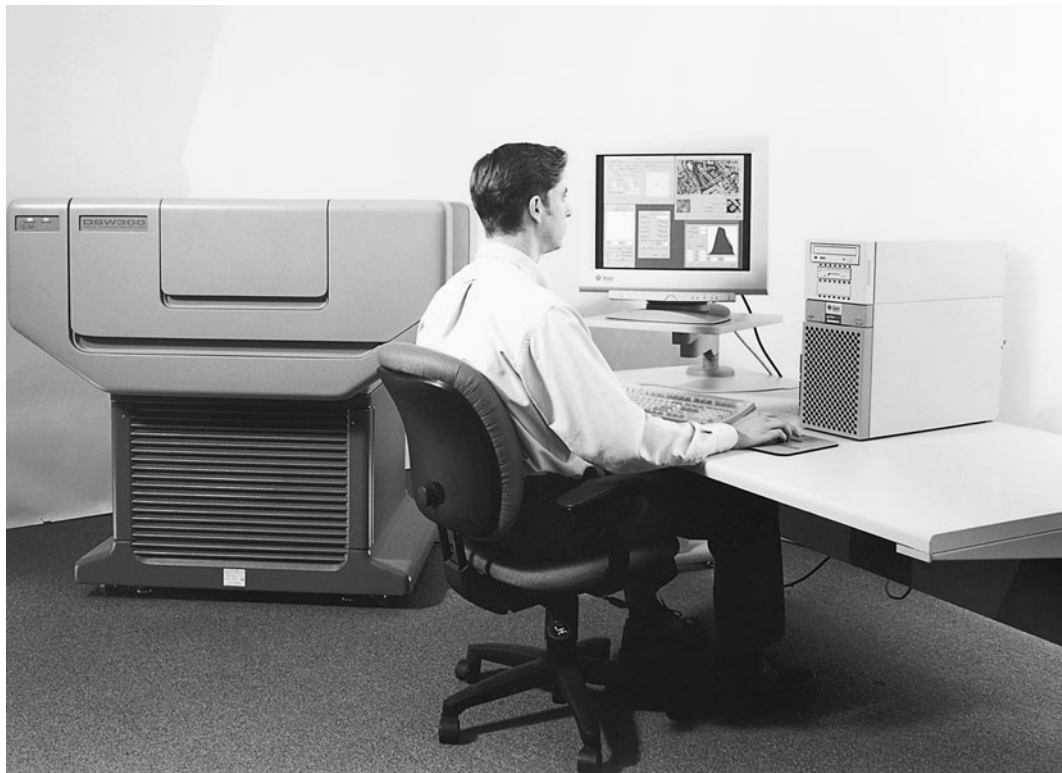
FIGURE 8.18 DSW300 scanner with Sun Ultra 60® host computer. This high-precision photogrammetric photo and film scanner has four elements: (a) movable xy cross carriage stage with flat film platen; (b) fixed array charge-coupled device (CCD) camera and image optics; (c) xenon light source and color scanning software; and (d) computer hardware, including storage. (Courtesy of Leica Geosystems Inc.)
