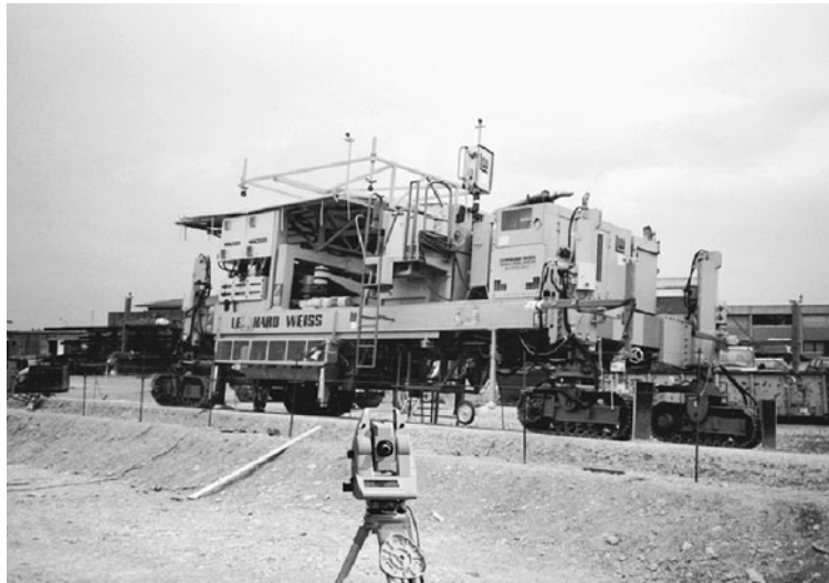
FIGURE 10.3 Paving-machine operation controlled by a motorized total station/radio control modem/PC computer instrumentation package. (Courtesy of Leica Geosystems Inc.)
