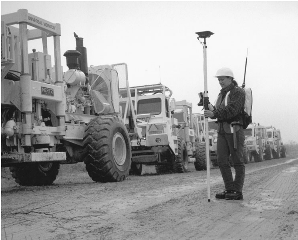
FIGURE 7.4 Trimble navigation total station GPS. Real-time positioning for a wide variety of applications. Features include GPS antenna and electronic field book at the adjustable pole; and receiver, radio, and radio antenna in the backpack. The receiver has been equipped with GPS processing software and the electronic field book has been equipped with the applications software (e.g., layout), thus permitting real-time data capture or layout. (Courtesy of Trimble Navigation, Sunnyvale, CA)
