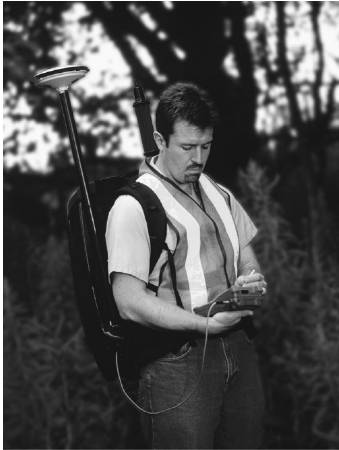
FIGURE 7.2 Combined IMU and RTK unit (see Section 8.11.4) carried in a backpack. This unit continues to determine position even when GPS signals are blocked by tree canopy or other obstructions. (Courtesy of Applanix Corp., Richmond Hill, Ontario)
