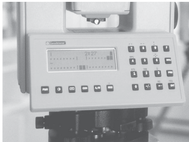
FIGURE 5.24 (a) Geodimeter 4400 base station. A total station equipped with servomotors controlling both the horizontal and vertical circle movements. Can be used alone as a conventional total station or as a robotic base station controlled by the remote-positioning unit (RPU) operator. (b) Geodimeter keyboard showing in-process electronic leveling. Upper cursor can also be centered by finally adjusting the third leveling screw.
