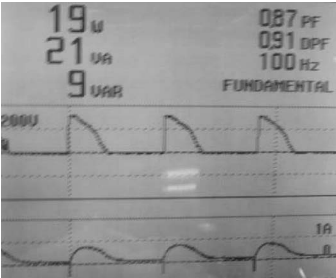
FIGURE 4.22 PF with input voltage 115 V and output voltage 80 V.
