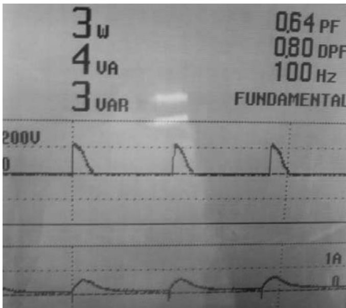
FIGURE 4.20 PF with input voltage 230 V and output voltage 80 V.
