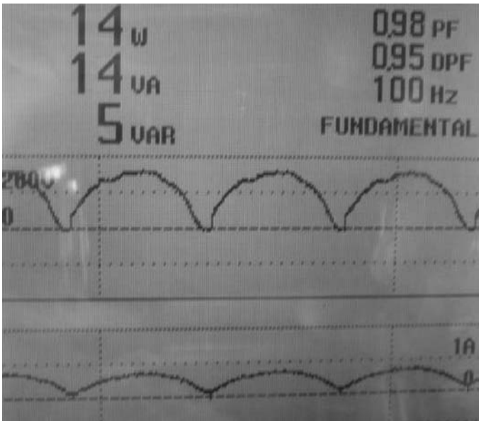
FIGURE 4.24 PF with input voltage 115 V and output voltage 103 V.
