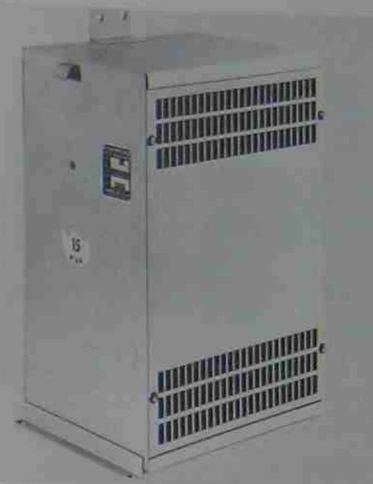
Figure 10.15 Single-phase dry-type transformer, type AA, rated at 15 kVA, 600 V/240 V, 60 Hz, insulation class 150°C for indoor use. Height: 600 mm; width: 434 mm; depth: 230 mm; weight: 79.5 kg. (Courtesy of Hammond)
