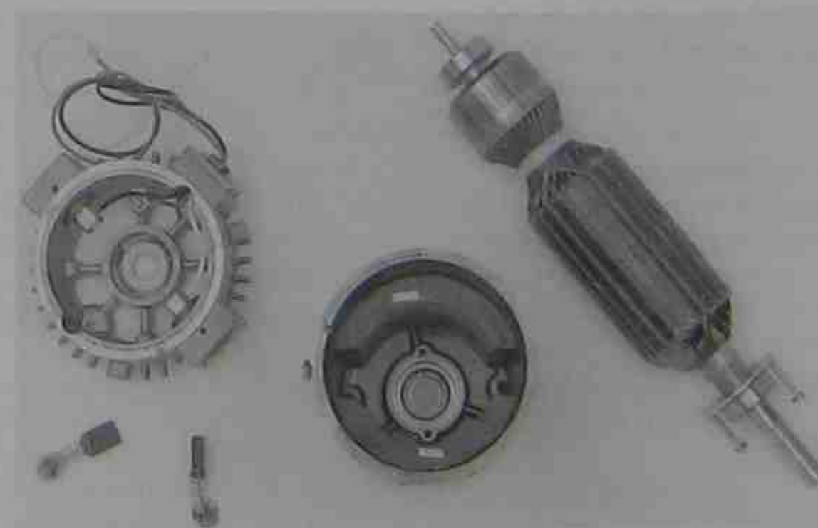
Figure 5.30 Permanent magnet motor rated 1.5 hp, 90 V, 2900 r/min, 14.5 A. Armature diameter: 73 mm; armature length: 115 mm; slots 20; commutator bars: 40; turns per coil: 5; conductor size: No. 17 AWG, lap winding. Armature resistance at 20°C: 0.34 Ω. (Courtesy of Baldor Electric Company)
