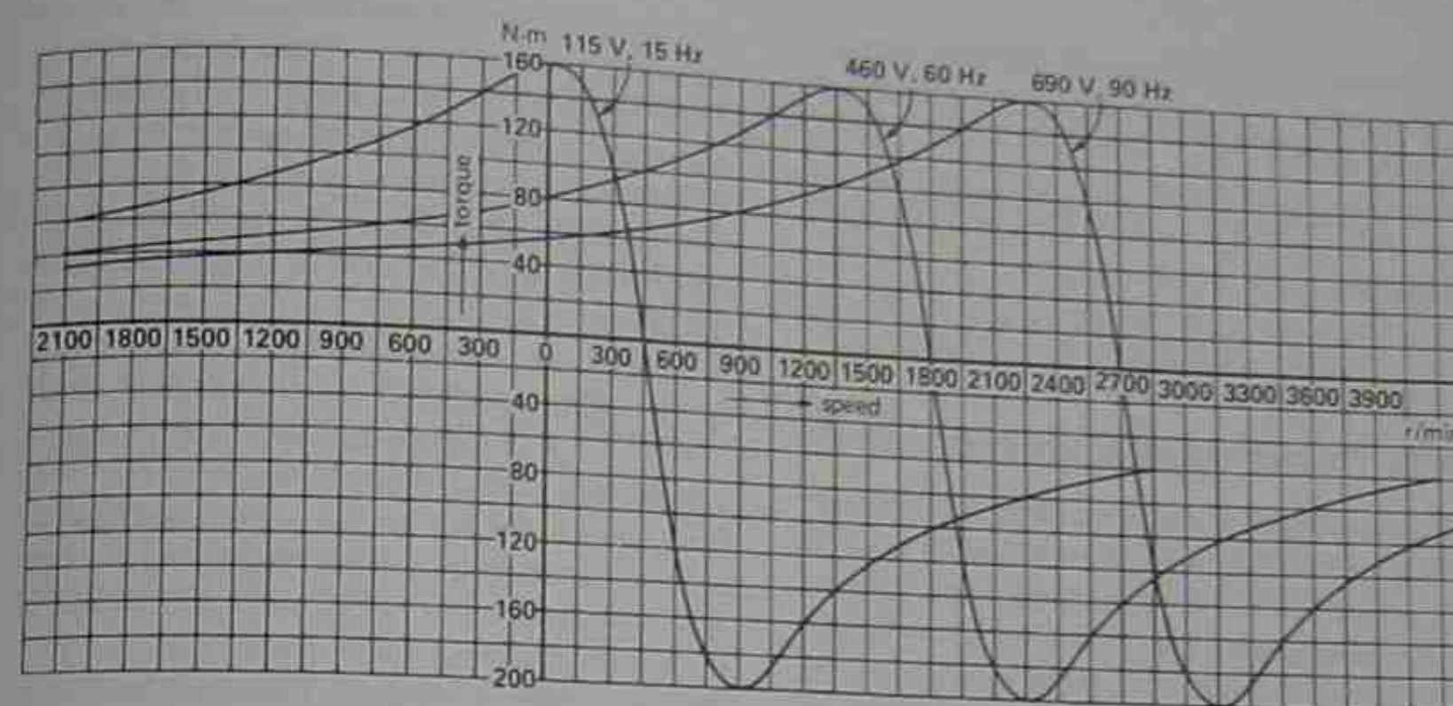
Figure 20.40 Torque-speed curve at three different frequencies and voltages.
