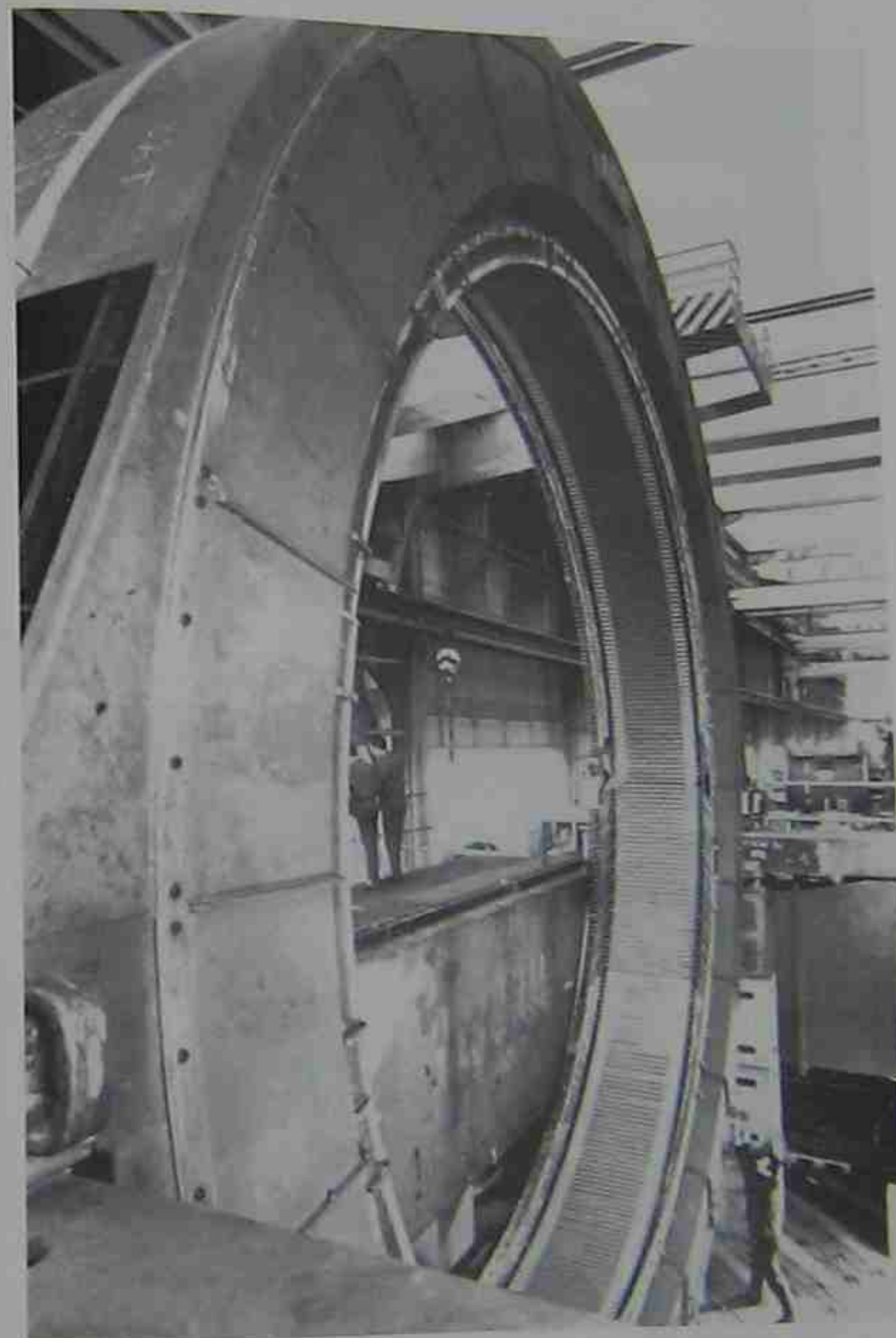
Figure 23.12a Stator of a 3-phase synchronous motor rated 6400 kW (8576 hp), 15 r/min, 5.5 Hz, 80^\circ\text{C} used to drive a ball-mill in a cement factory. The stator is connected to a 50 Hz cycloconverter, whose output frequency is variable from zero to 5.5 Hz. Internal diameter of stator: 8000 mm; active length of stacking: 950 mm; slots: 456. (Courtesy of ABB)
