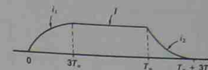
Figure 19.20d Real current pulse.
