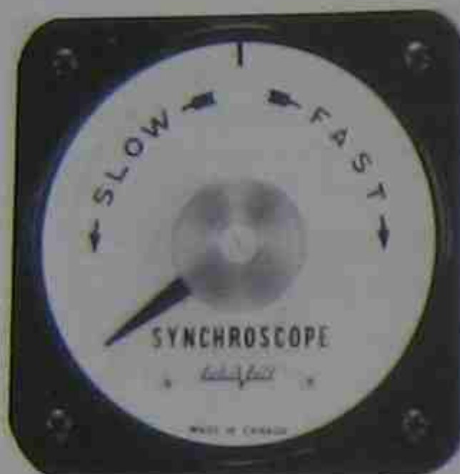
Figure 16.24 Synchroscope. (Courtesy of Lab-Volt)
