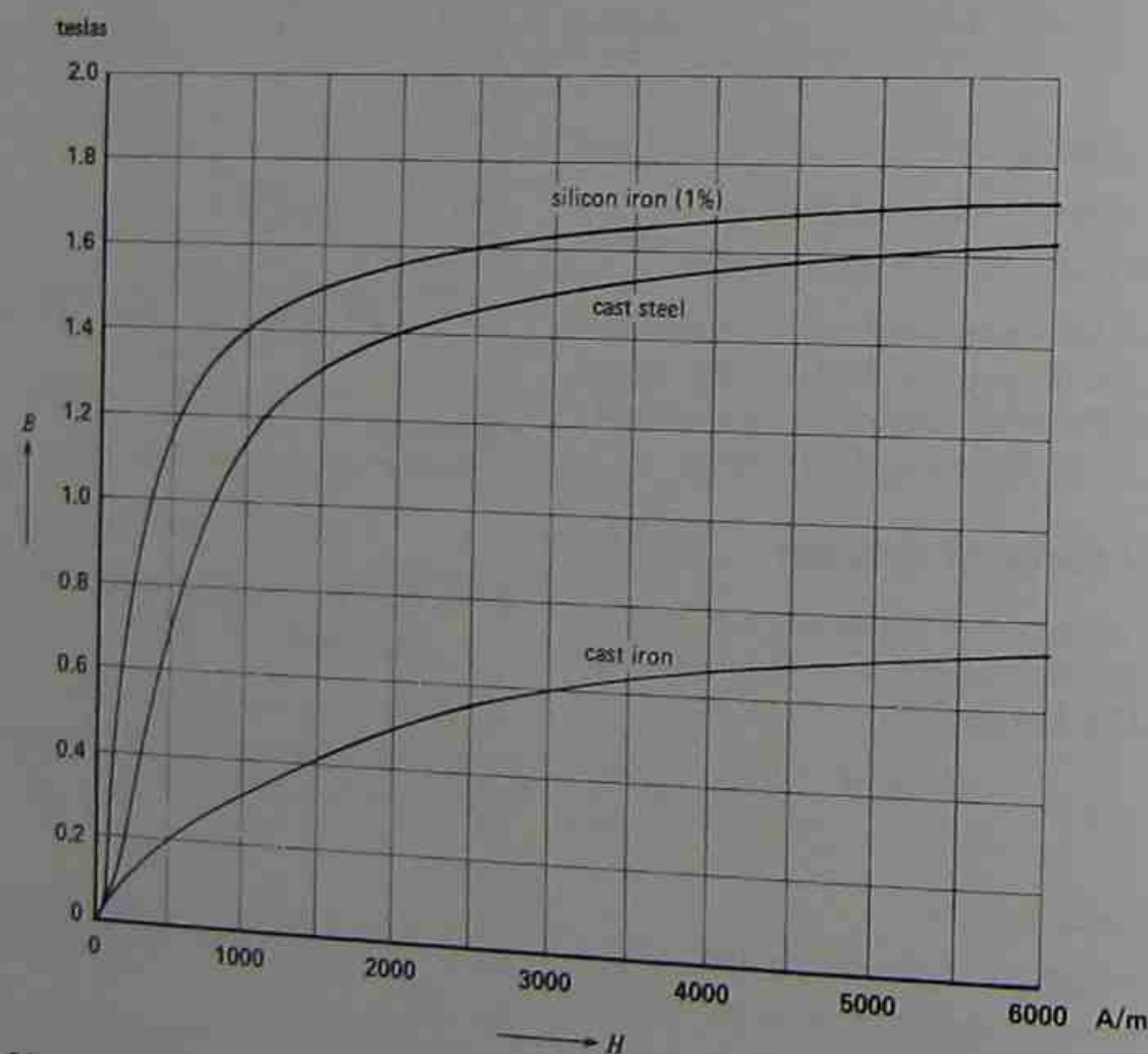
Figure 2.26 B - H saturation curves of three magnetic materials.
