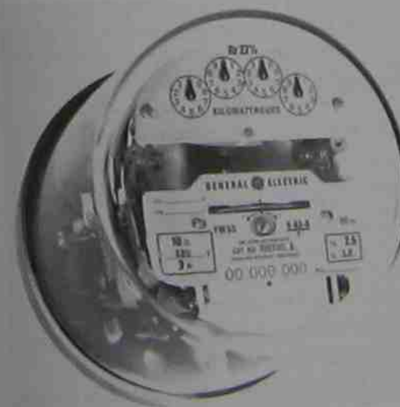
Figure 27.15 Watt-hourmeter for a 3-phase, 3-wire circuit. (Courtesy of General Electric)
