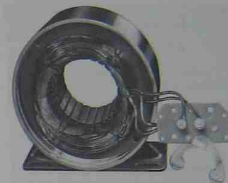
Figure 18.4 Main and auxiliary windings in a 2-pole single-phase motor. The stationary contact in series with the auxiliary winding opens when the centrifugal switch, mounted on the shaft, reaches 75 percent of synchronous speed.
