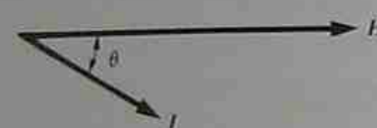
Figure 2.18 Phasor I lags behind phasor E by an angle of \theta degrees.
