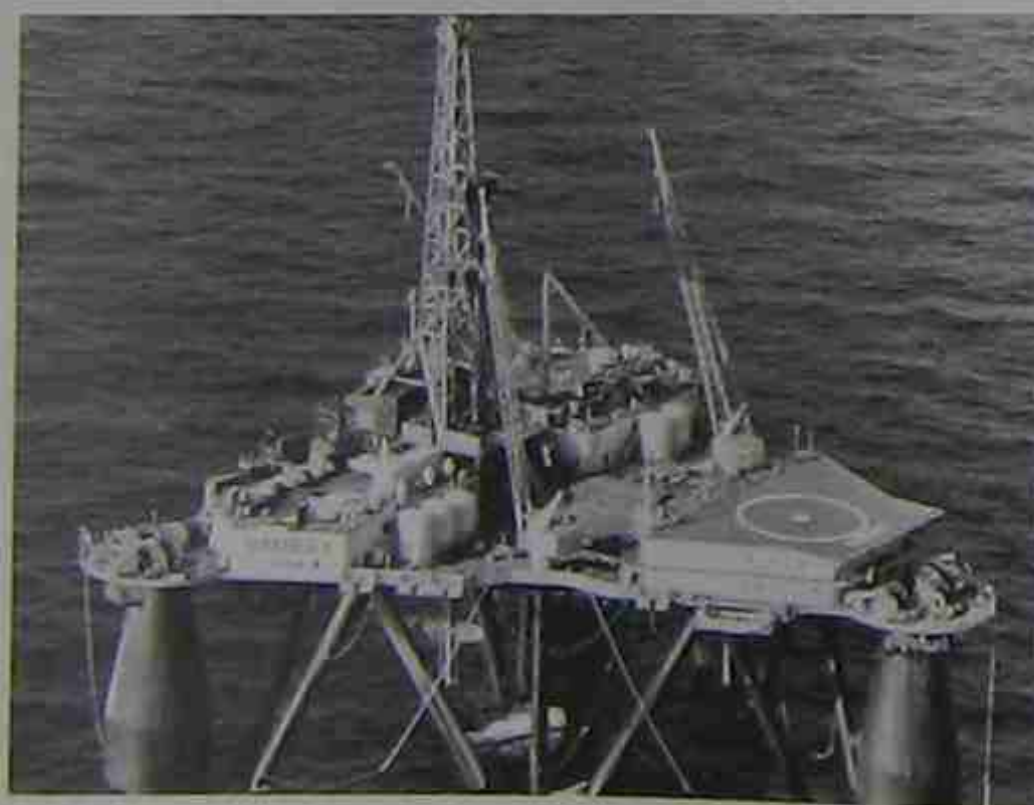
Figure 16.25 This floating oil derrick provides its own energy needs. Four diesel-driven generators rated 1200 kVA, 440 V, 900 r/min, 60 Hz supply all the electrical energy. Although ac power is generated and distributed, all the motors on board are thyristor-controlled dc motors. (Courtesy of Siemens)
