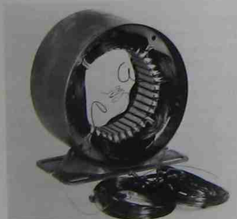
Figure 18.2c Four poles of the auxiliary winding straddle the main winding. (Courtesy of Lab-Volt)
