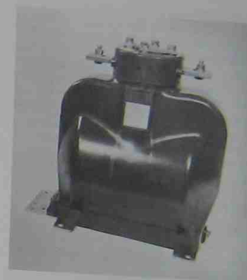
Figure 11.17 Epoxy-encapsulated current transformer rated 50 VA, 400 A/5 A, 60 Hz and insulated for 36 kV. (Courtesy of Montel, Sprecher & Schuh)
