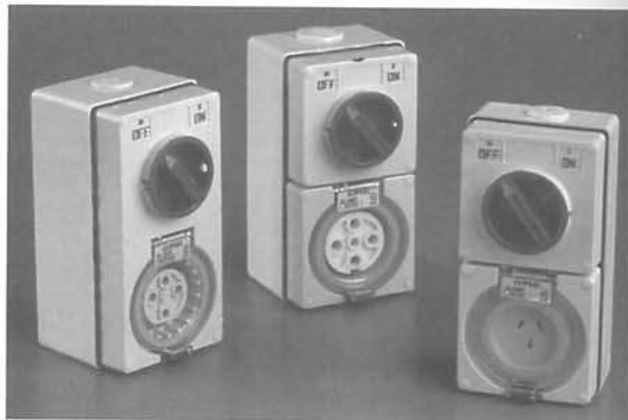
Fig. 5.27(c) 'Weatherproof/hoseproof' IP56 switch and socket outlet designed on a modular system. Cases are PVC, lids polycarbonate WILCO PRODUCTS
