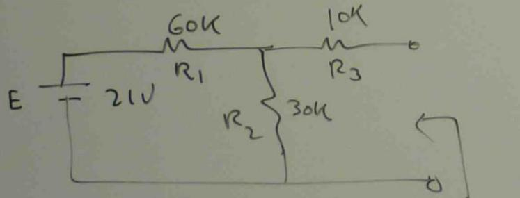
$$V_{R2} = E \times \frac{R_2}{R_1 + R_2} = 21 \times \frac{30}{60+30} = 7 \text{ V}$$
