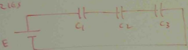
$$\frac{1}{C_T} = \frac{1}{C_1} + \frac{1}{C_2} + \frac{1}{C_3}$$
