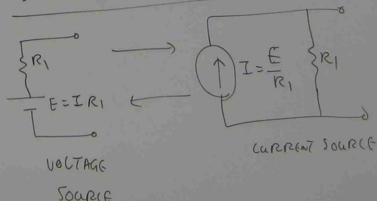
Ex CONVERT THE VOLTAGE SOURCE OF GIVEN FIGURE TO A CURRENT SOURCE AND CALCULATE THE CURRENT THROUGH THE  $4\ \Omega$  LOAD
