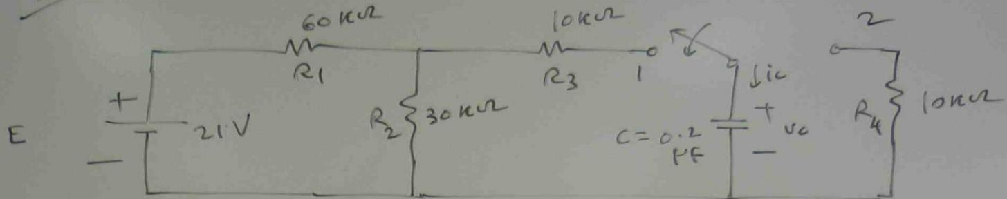
(a) FIND THE MATHEMATICAL EXPRESSION FOR THE TRANSIENT BEHAVIOUR OF THE VOLTAGE  $v_c$  AND THE CURRENT  $i_c$  FOLLOWING THE CLOSING OF THE SWITCH POSITION 1 AT  $t = 0$  SEC.
