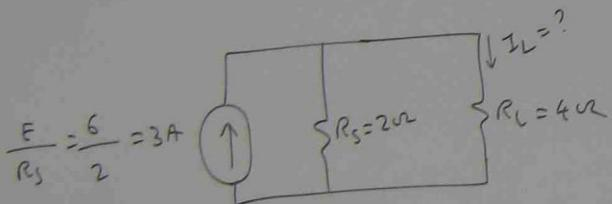
$$I_L = I_T \times \frac{R_S}{R_S + R_L}$$
