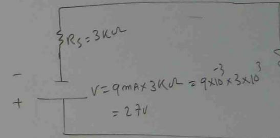
$$V = 9\text{ mA} \times 3\text{ k}\Omega = 9 \times 10^{-3} \times 3 \times 10^3 = 27\text{ V}$$
