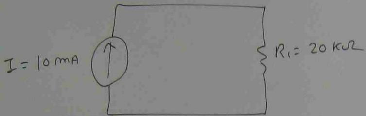
$$\begin{aligned}V_s &= IR_L \\&= 10 \text{ mA} \times 20 \text{ K} \\&= 10 \times 10^{-3} \times 20 \times 10^3 \\&= 200 \text{ V}\end{aligned}$$
