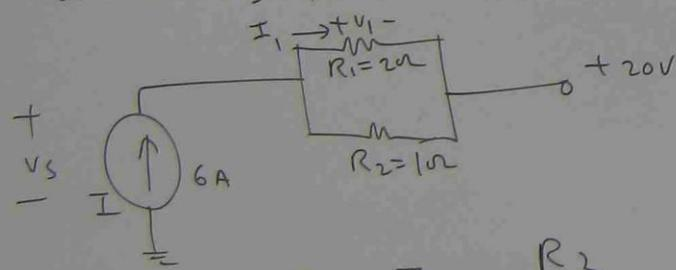
$$I_1 = I \times \frac{R_2}{R_1 + R_2}$$
