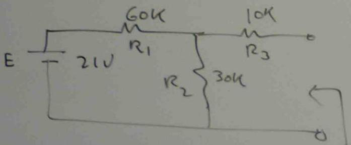
$$V_{R2} = E \times \frac{R_2}{R_1 + R_2} = 21 \times \frac{30}{60+30} = 7V$$
