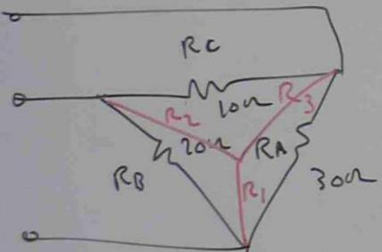
$$R_L = \frac{R_A \times R_B}{R_A + R_B + R_C} = \frac{30 \times 20}{30 + 20 + 10}$$
