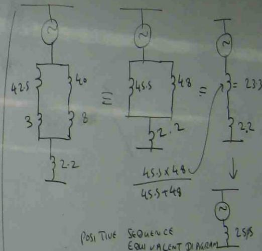
IN THIS PROBLEM, THE SAME  $Z$ . IMPEDANCE IS GIVEN FOR BOTH POSITIVE, NEGATIVE AND ZERO SEQUENCE. IF THE DIFFERENT POSITIVE, NEGATIVE AND ZERO SEQUENCE IMPEDANCES ARE GIVEN, USE RESPECTIVE VALUE FOR RESPECTIVE EQUIPMENT CIRCUIT
