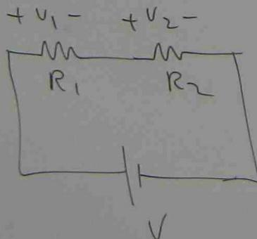
$$V_1 = V \times \frac{R_1}{R_1 + R_2}$$
