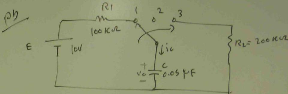
(a) FIND THE MATHEMATICAL EXPRESSION FOR THE TRANSIENT BEHAVIOUR OF THE VOLTAGE ACROSS THE CAPACITOR IF THE SWITCH IS THROWN INTO POSITION 1 AT  $t = 0$  SEC.
