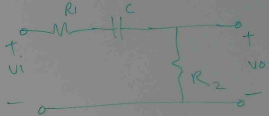
$$A_V = \frac{V_o}{V_i} = \frac{R_2}{R_1 + R_2} \left[ \frac{1}{1 - j \frac{f_c}{f}} \right]$$
