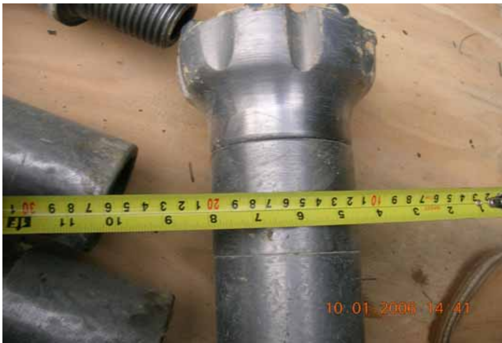
Figure 62: Size of drilling rig is checked before drilling
