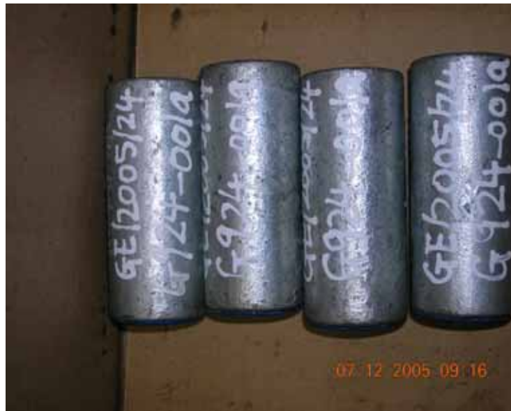
Figure 32: Coupler is used to connect the reinforcement
