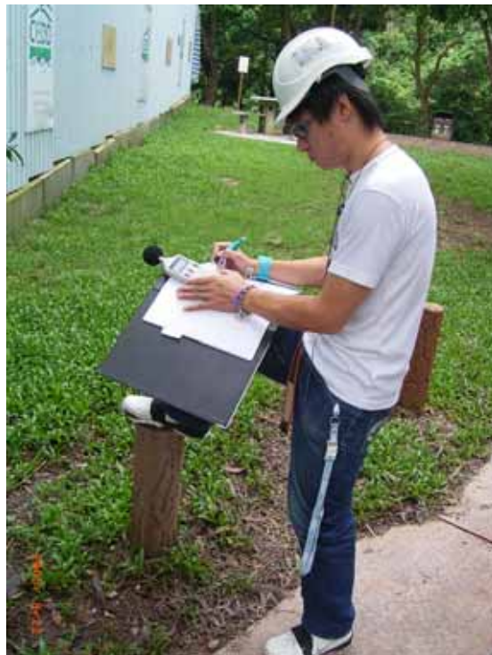
Figure 88: Noise Assessment was conducted by Contractor
