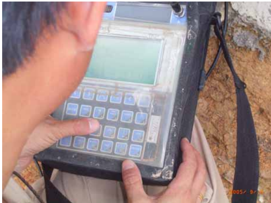
Figure 68: TDR test in progress
