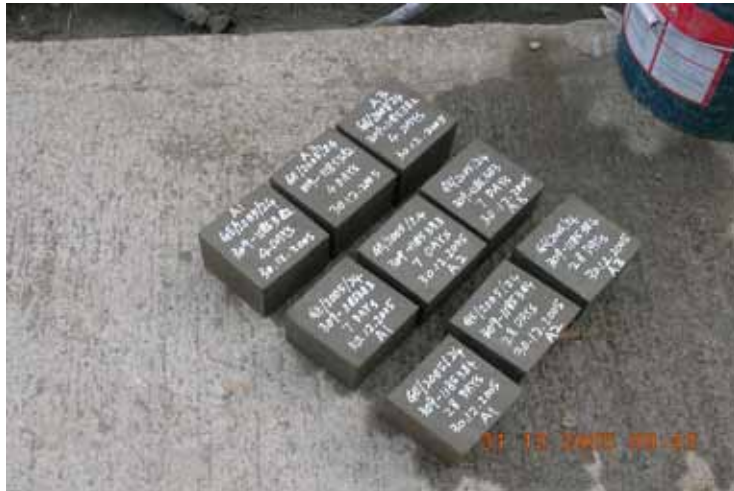
Figure 39: Cement cube (100 mm 3 ) was prepared for testing
