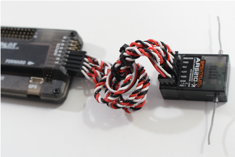
Figure 6-3. Our Spektrum receiver is plugged into the APM input on the bench.
