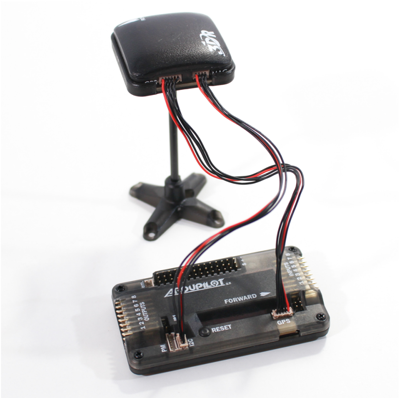
Figure 5-7. Our GPS and compass (magnetometer) plugged into the APM.
