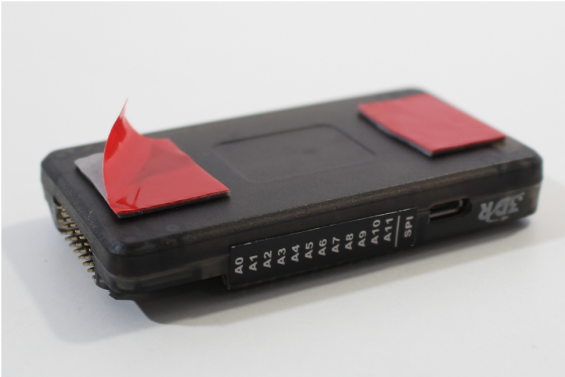
Figure 4-4. Cut your tape in half and place each portion at one end of the APM, then peel off the backing.
