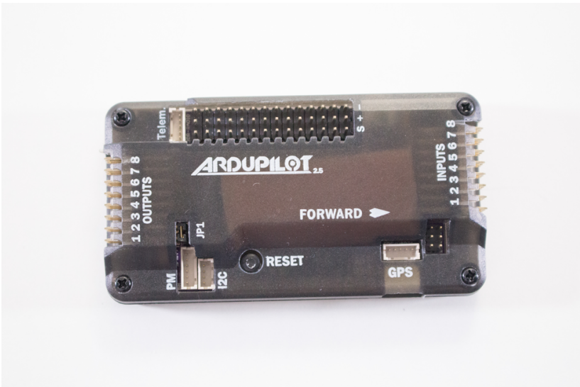
Figure 4-1. This flight controller has a built-in IMU and ports for external sensors.
