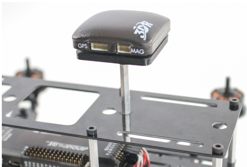
Figure 5-4. We like to keep things simple with this DIY GPS mast.
