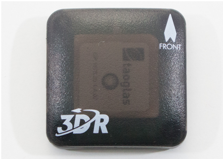
Figure 5-1. 3DR uBlox GPS unit with built-in compass.
