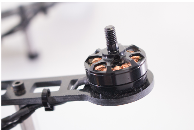
Figure 3-4. These 2204 motors are rated at 2300 kV and work with 5- or 6-inch props.
