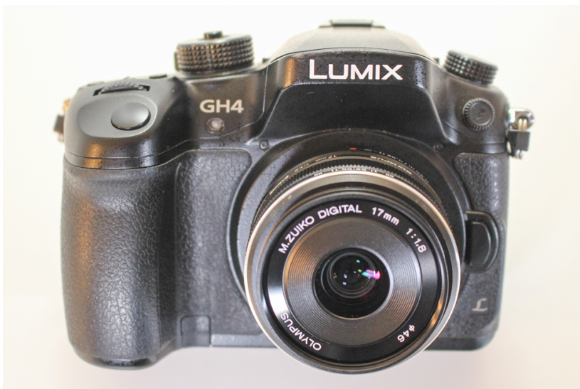
Figure 8-1. A very popular micro four thirds camera, the Lumix GH4 camera body with an Olympus 17-mm wide angle lens.
