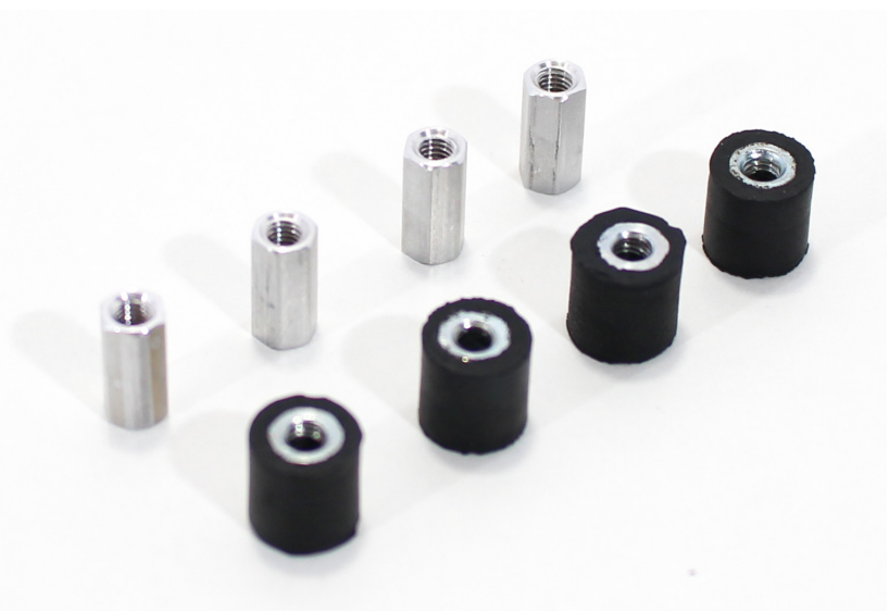
Figure 2-6. Standoffs—either aluminum for stiffness and longer life, or rubber for increased vibration isolation—are used to separate the two subframes.
