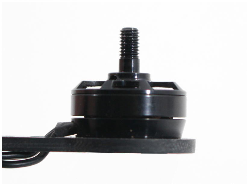
Figure 3-31. Our motor is sitting squarely on the boom ready to be attached.
