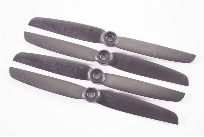
Figure 3-2. Two pushers and two tractors.
