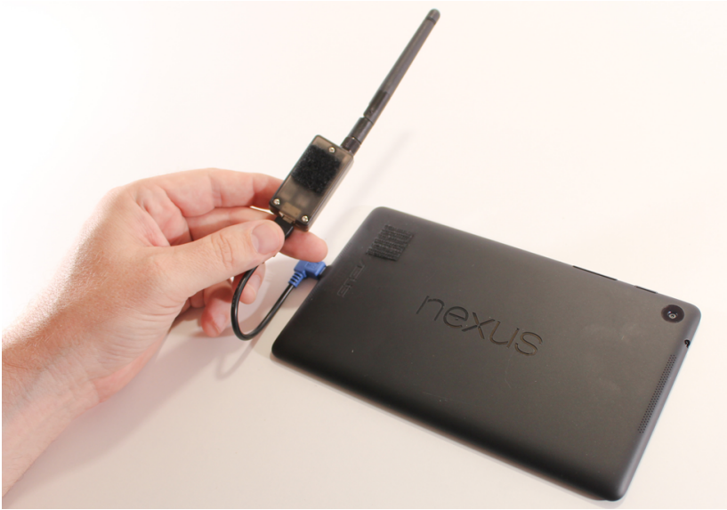
Figure 7-2. Velcro holds the telemetry radio on the back of our tablet while in use and allows for easy removal when we are not flying.
