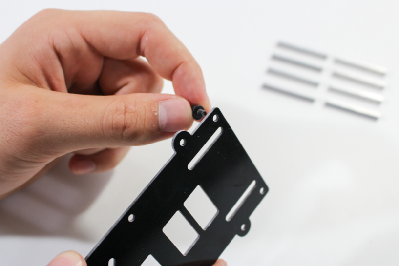
Figure 2-14. Pushing the 5-mm screw through the standoff mounting holes on plate D.
