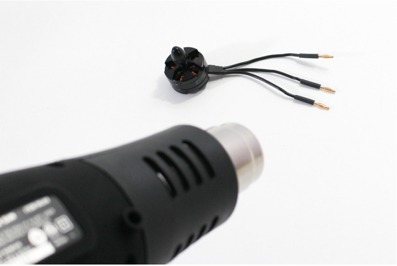
Figure 3-16. Using our heat gun to shrink our tubing for insulation purposes.
