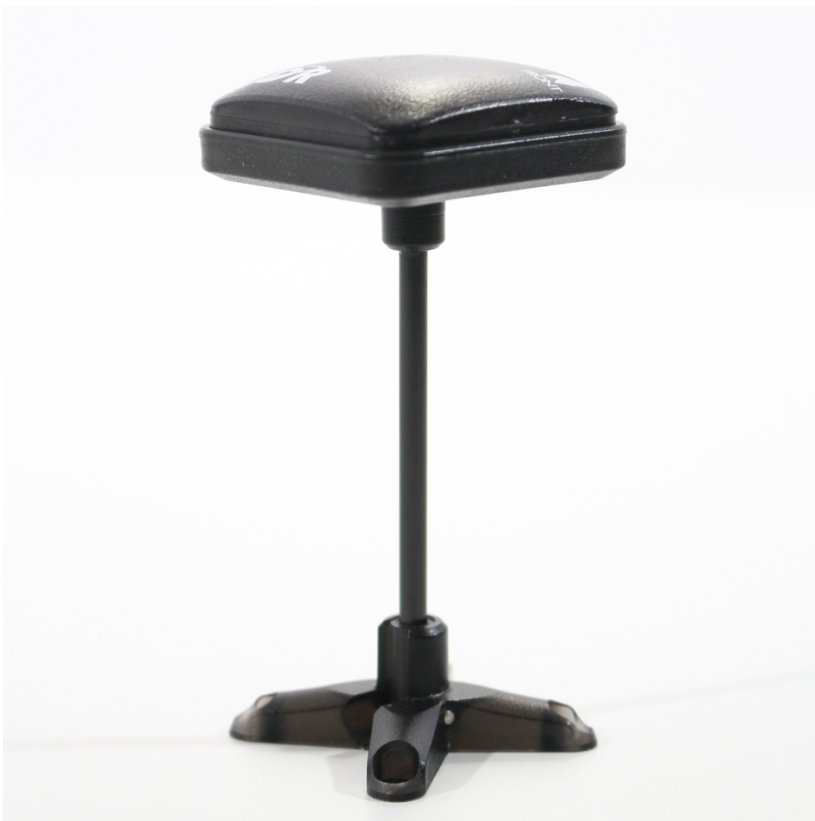
Figure 5-3. 3DR makes a nice mast for the uBlox GPS.
