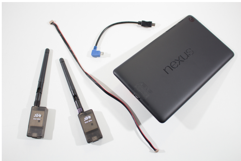
Figure 7-1. This Android tablet can be used a ground station with the addition of telemetry radios and a free app.
