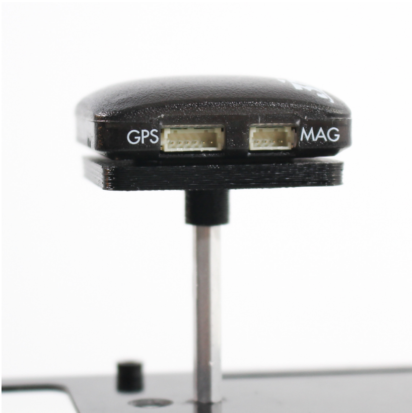
Figure 5-6. The two ports on the side of our GPS puck.
