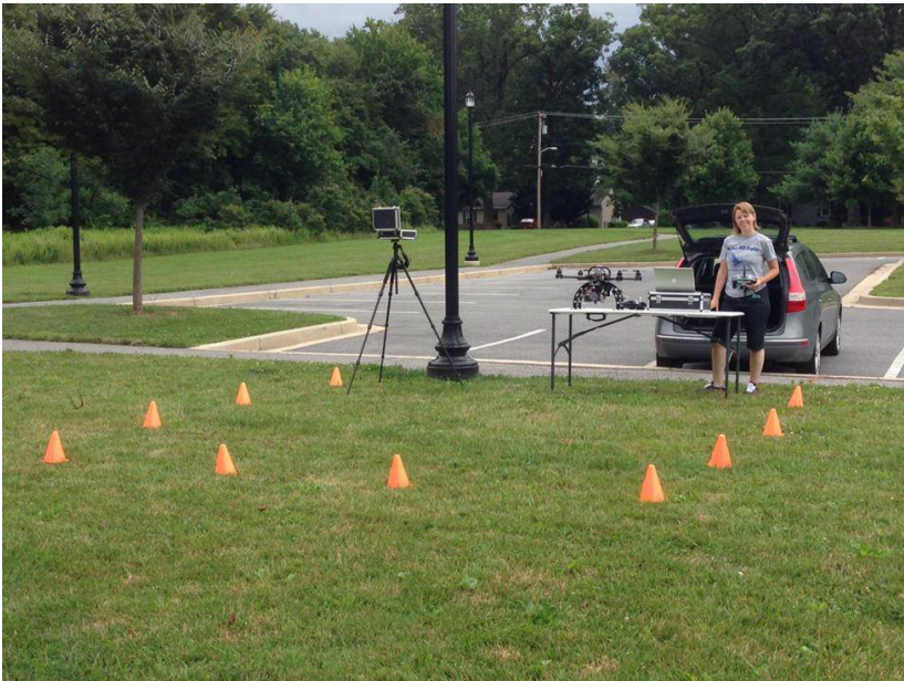
Figure 10-1. Always keep a safety zone around your aircraft during takeoff and landing.
