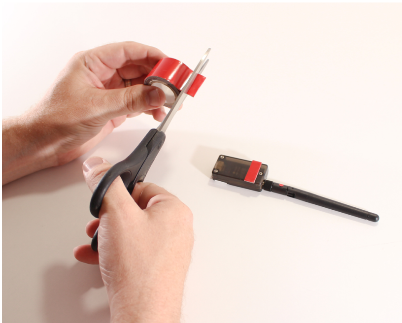
Figure 7-3. Double-sided foam tape can be used to fasten the radio to the air frame.
