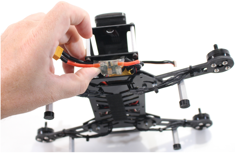
Figure 5-10. Getting our battery monitor into position and ready to be fastened to the frame.
