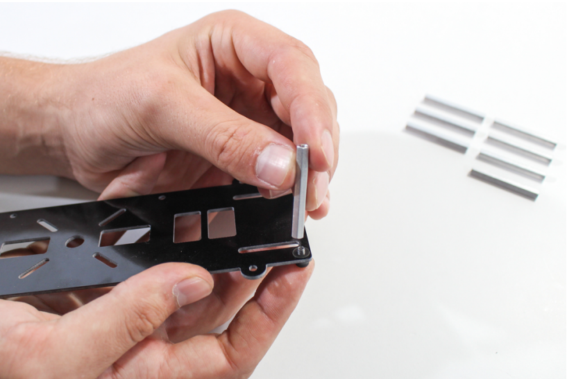
Figure 2-15. Threading the first 37-mm standoff on the back of our mounting screw.
