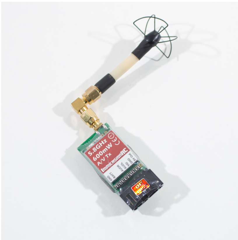
Figure 8-3. 5.8 GHz video transmitter with optional cloverleaf antenna and right angle.
