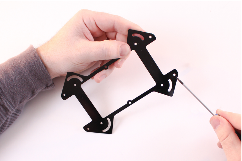
Figure 2-7. Pointing out the standoff mounting holes on plate B of the dirty frame.
