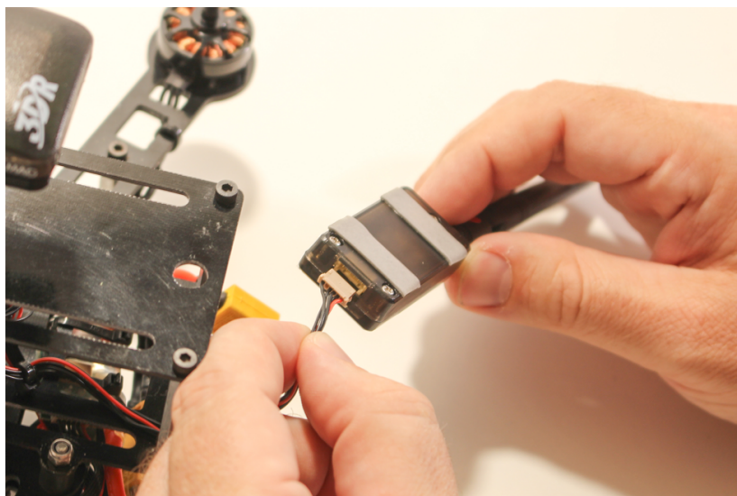
Figure 7-4. Plugging in the telemetry radio will be much easier if done before it's mounted to the frame.
