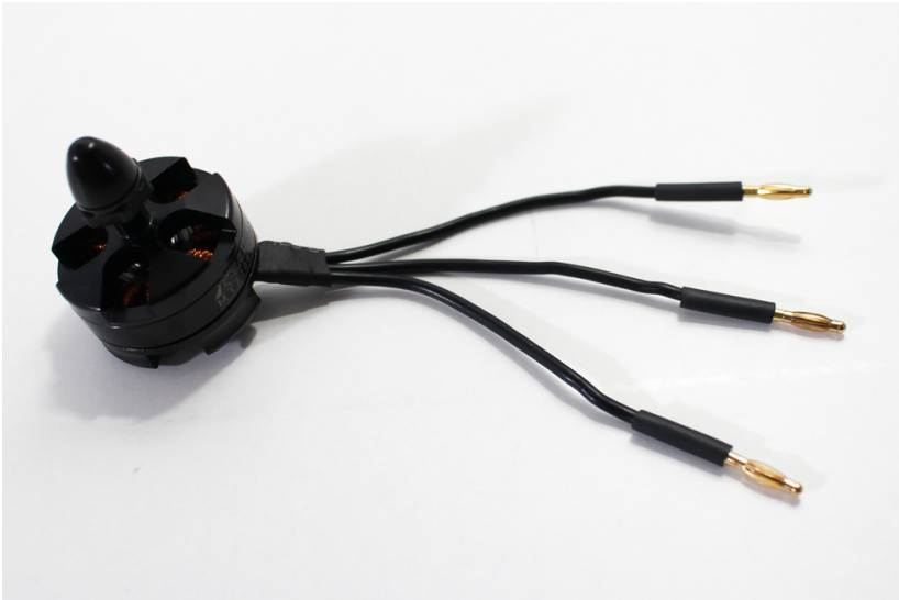
Figure 3-15. Heat shrink is in place and ready for the heat gun.
