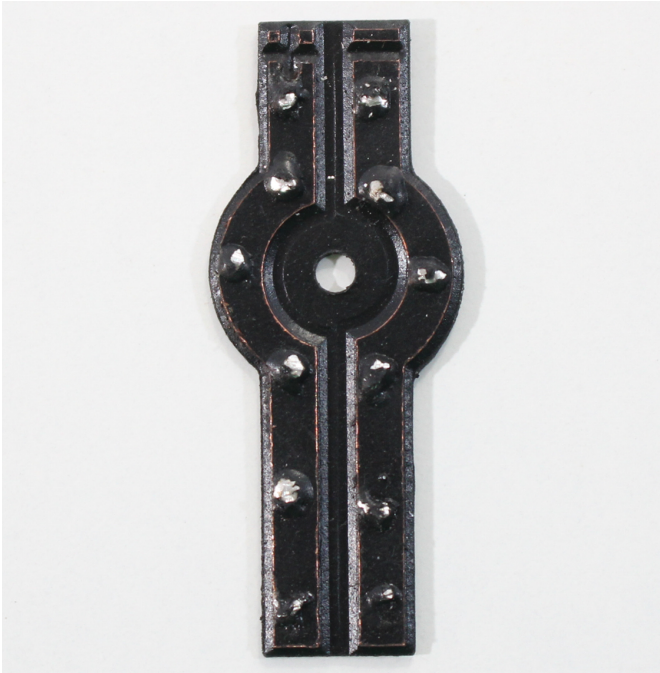
Figure 3-9. This is what our PDB looked like—we tinned a few solder spots and added liquid tape for a layer of insulation.
