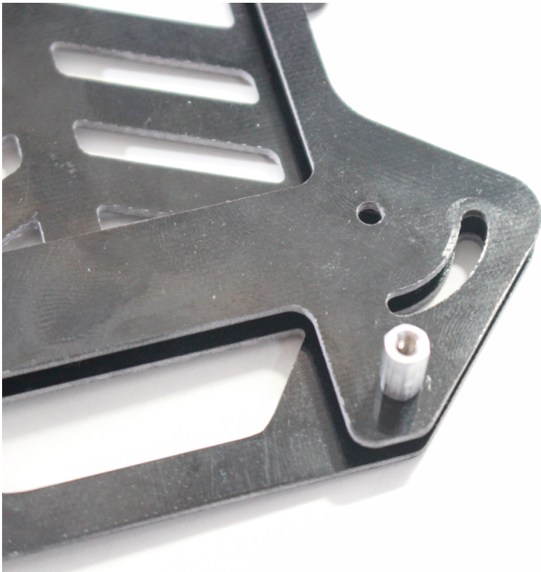
Figure 2-10. Rear boom mounting holes (notice the anchor hole just above the folding slot).
