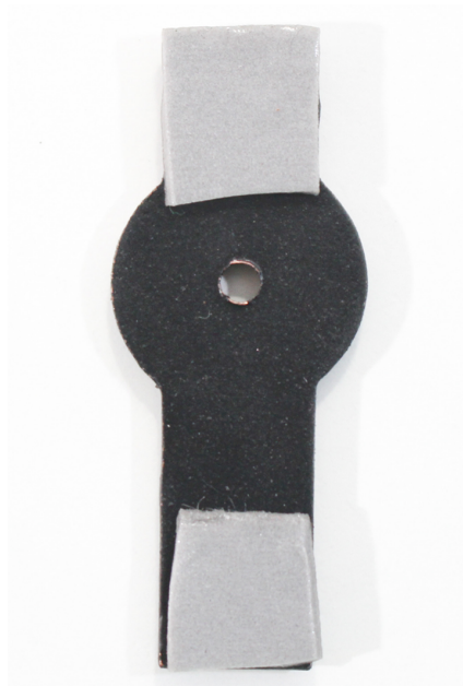
Figure 3-10. Applying double-sided tape to the back side of the PDB.
