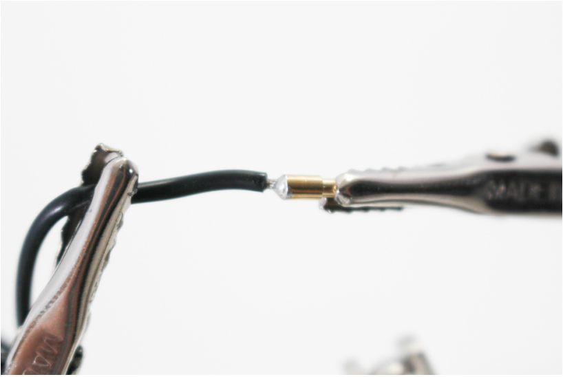
Figure 3-14. Our solder is cooling while being held in place with the third hand.
