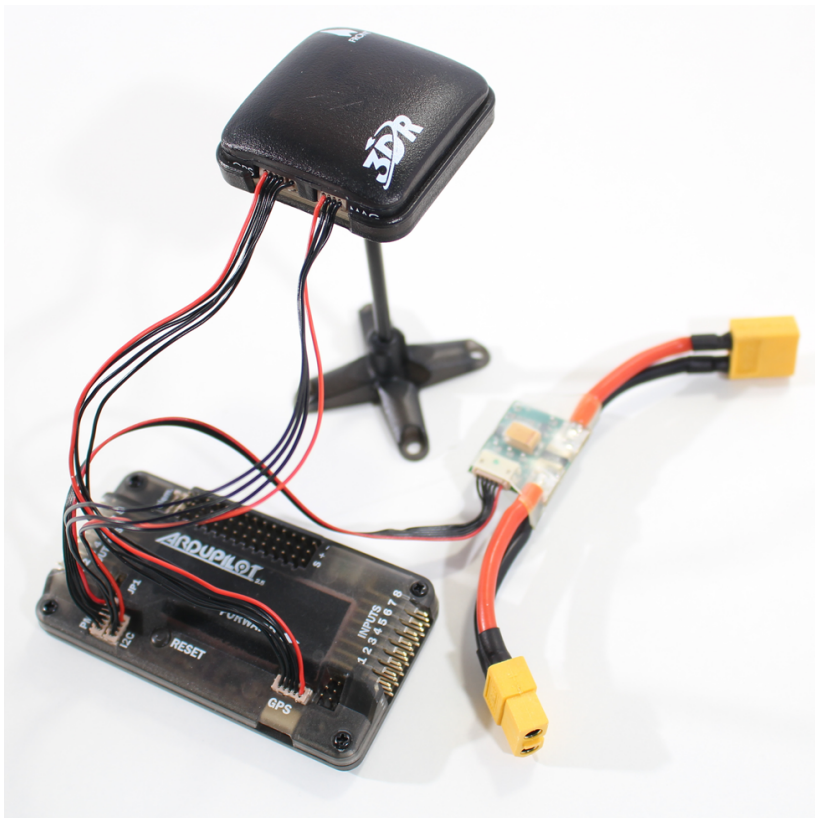
Figure 5-8. Our battery monitor plugged in on the bench, speaking to the APM over a 6-position cable that plugs into the PM port.
