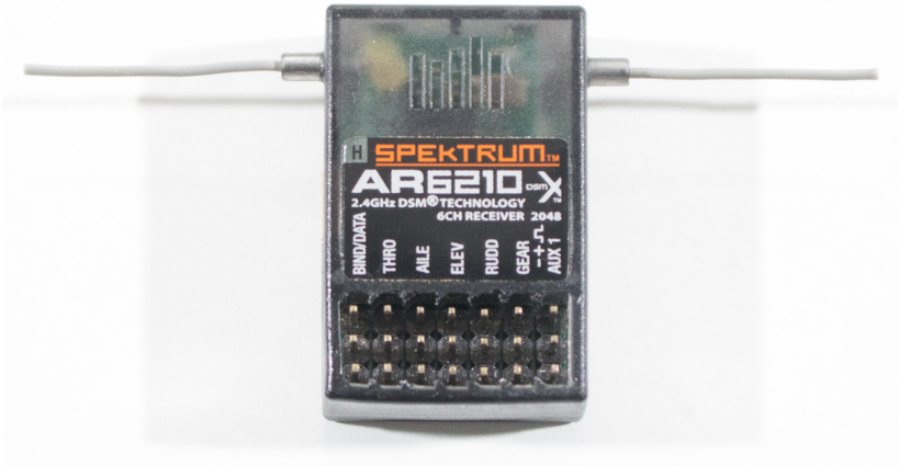
Figure 6-2. Six-channel receiver by Spektrum.
