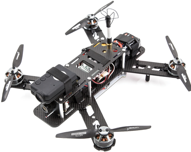
Figure 2-4. QAV250 with 5X3 carbon fiber props.
