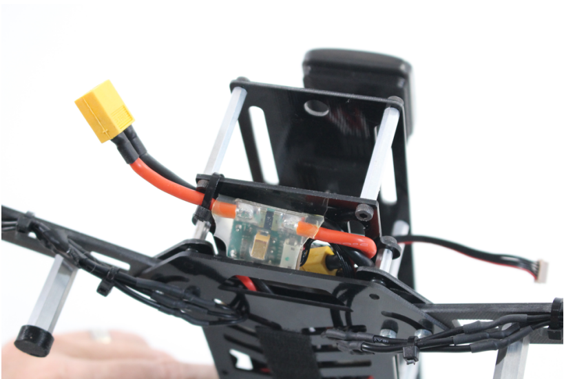
Figure 5-11. The new battery lead is accessible to the flight battery.
