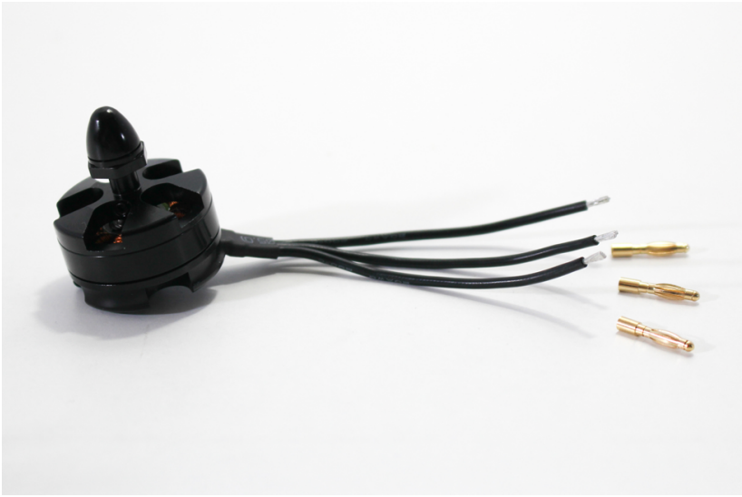
Figure 3-12. The motor leads are stripped, tinned, and ready to take the male bullet connectors.
