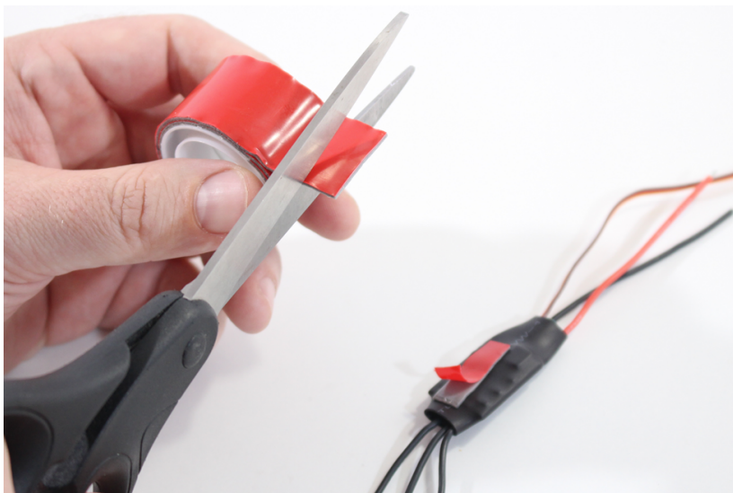
Figure 3-22. Apply a small strip of double-sided tape of the flat-test side of the ESC.
