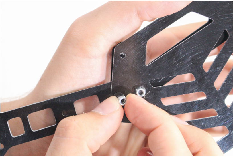
Figure 2-13. Placing the nuts on the bottom of the frame.
