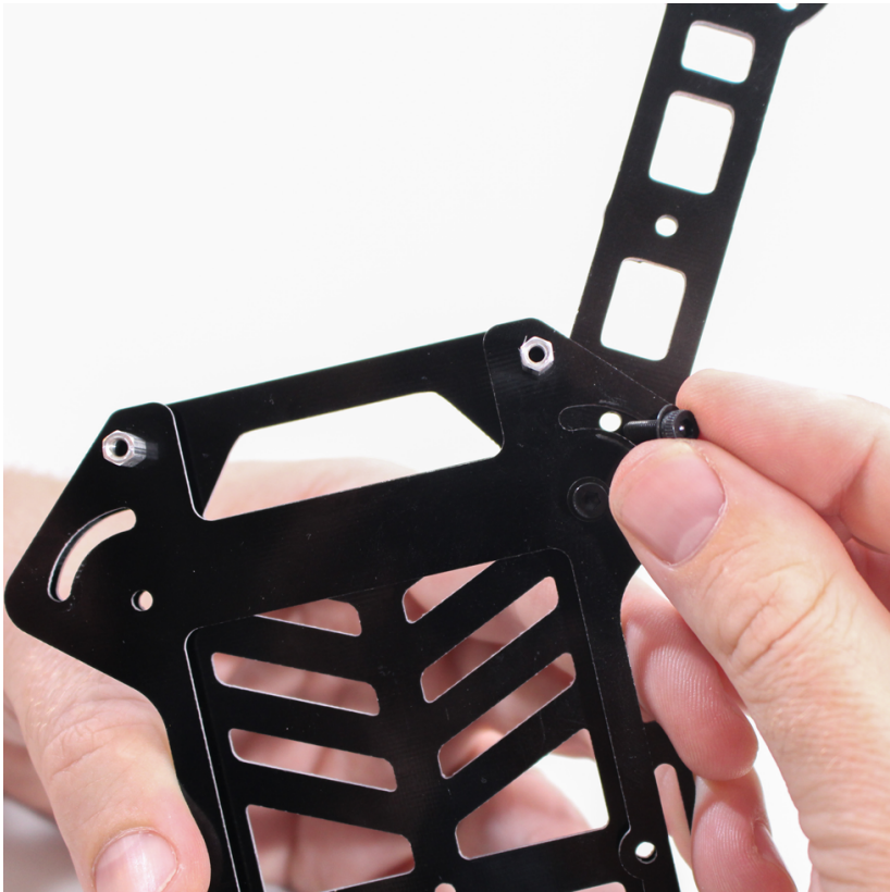
Figure 2-12. Pushing the second screw through the mounting holes.
