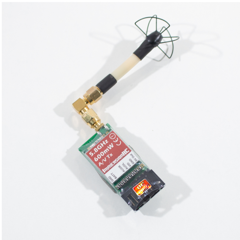
Figure 12-1. 5.8 GHz video transmitter with a right-angle adapter and right-handed Skew Planer antenna.
