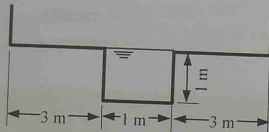
*Case a:*  $S_0=0.001$ ,  $n=0.02$ , estimate the discharge in the channel
