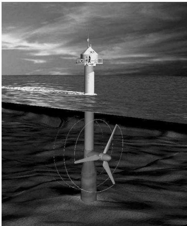
Figure 7.2-22 Artist's impression of the Lynmouth turbine being installed in the Bristol Channel. Illustration reproduced with the kind permission of Marine Current Turbines Ltd.
