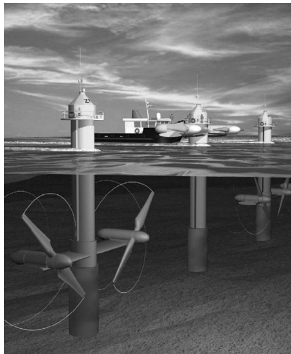
Figure 7.2-24 Artist's impression of an array of twin rotor tidal current devices. Illustration reproduced with the kind permission of Marine Current Turbines Ltd.
