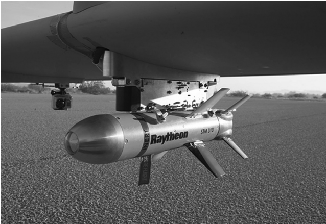
Figure 7.5 Installation of Pyros under the UAV platform.
