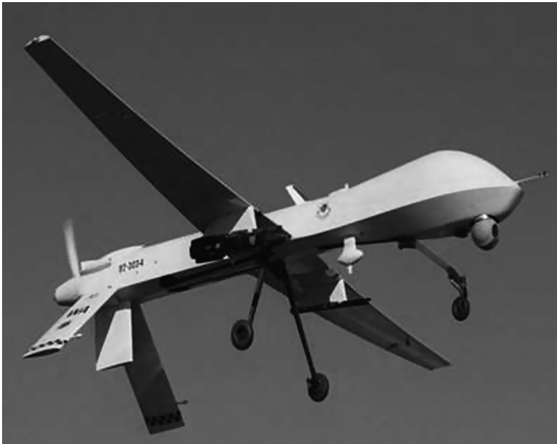
Figure 2.5 Critical elements of the hunter-killer MQ-9 Predator equipped with multiple sensors and laser guided missiles.
