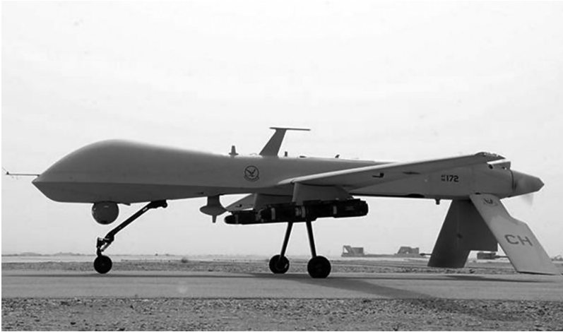
Figure 2.4 Critical elements and EO/IR sensors associated with MQ-1 Predator UAV for missile-hunting missions.
