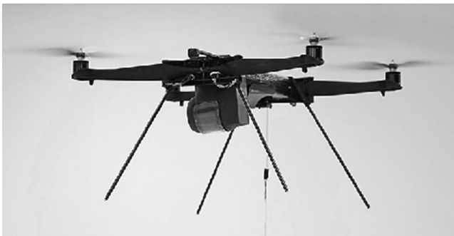
Figure 5.1 Tactical drone capable of flying over long distances using a tether to provide communication link and power to the tactical drone.
