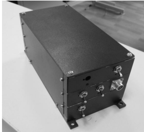
Fig. 6.19 Breadboard model of the integrated inertial-satellite navigation system
