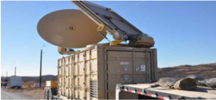
Figure 9-9 High-Power Microwave Weapon to Destroy or Disable Swarms of Unmanned Aircraft
