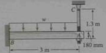
Figure 10.37 Beam in Example 10.7.
