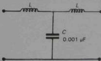
Fig. 7.6. One section of the pulse-forming network
