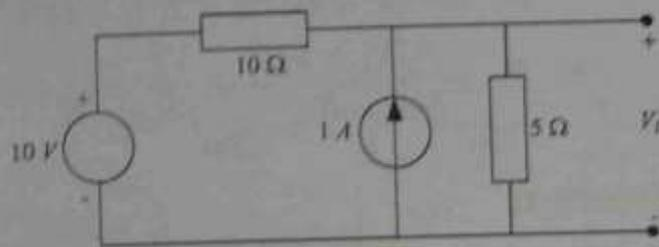
Figure 3.10: An electric circuit containing multiple sources.
