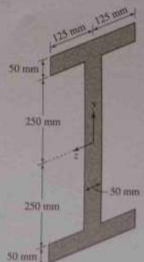
Figure 3.46 Beam cross section in Example 3.16.
