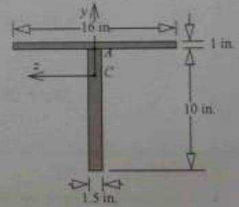
Figure 6.19 T cross section in Example 6.5.
