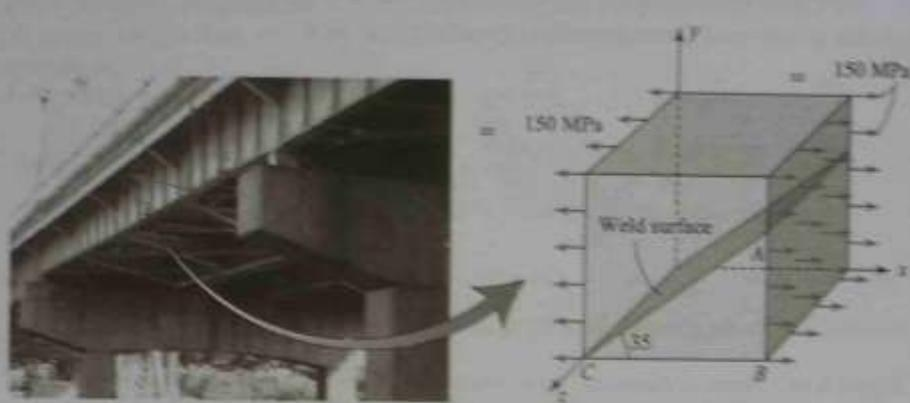
Figure 8.3 Stress cube at a point on a bridge.
