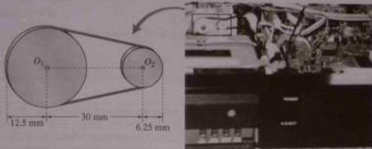
Figure 2.10 Belt and pulley in a VCR.
