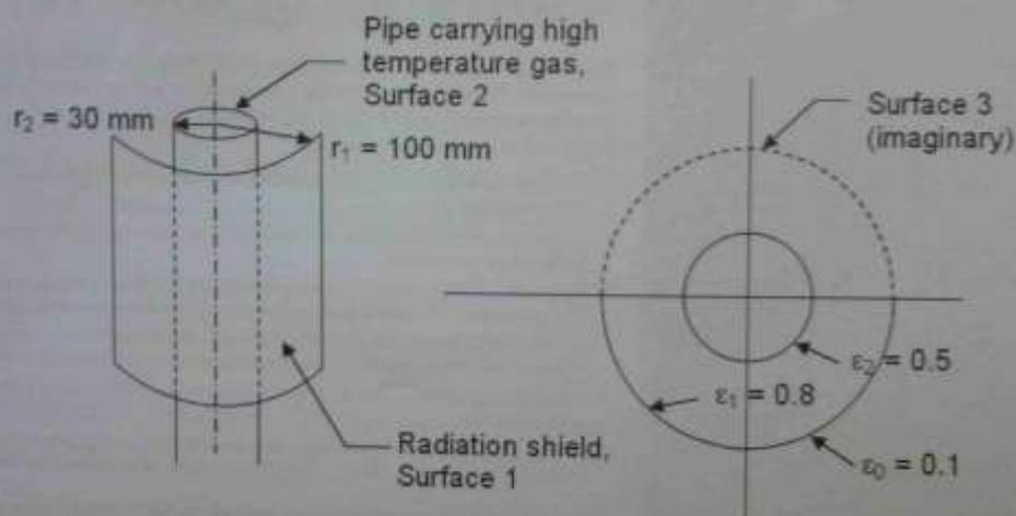
Figure 4.4 Radiation shield - Example 4.2
